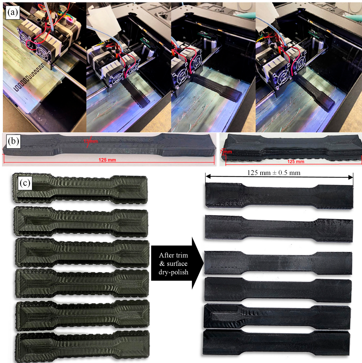
Figure 2. (a) Typical 3D printing strategy used, (b) faulty-produced specimens with distortion and disbonding, (c) optimally produced specimens using the final 3D printing parameter settings.
