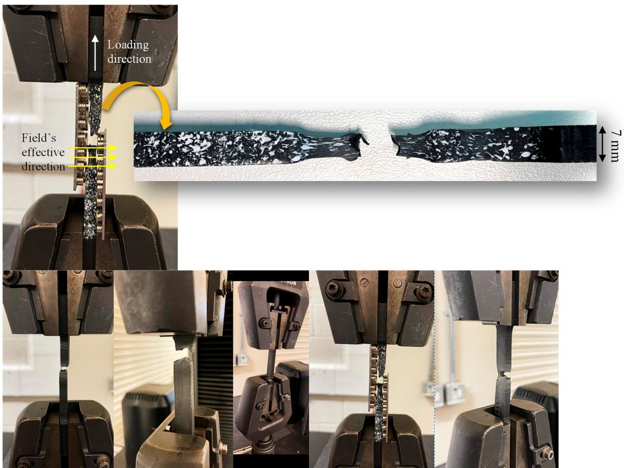
Figure 6. Typical specimen with speckled surface (for DIC measurements) at its ultimate failure point.
