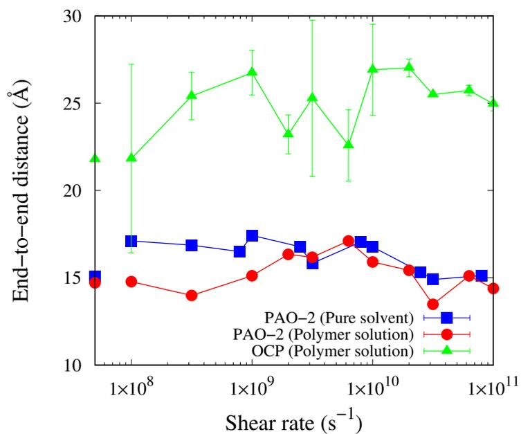
**Figure A7:** The end-to-end distance ( $R_e$ ) of PAO-2 and OCP in pure solvent and polymer solution as a function of shear rate at 313 K. The data points on the y-axis show the values of  $R_e$  at zero shear rate. The data shows that  $R_e$  of OCP increases as a function of shear rate whereas that of PAO-2 remains constant.
