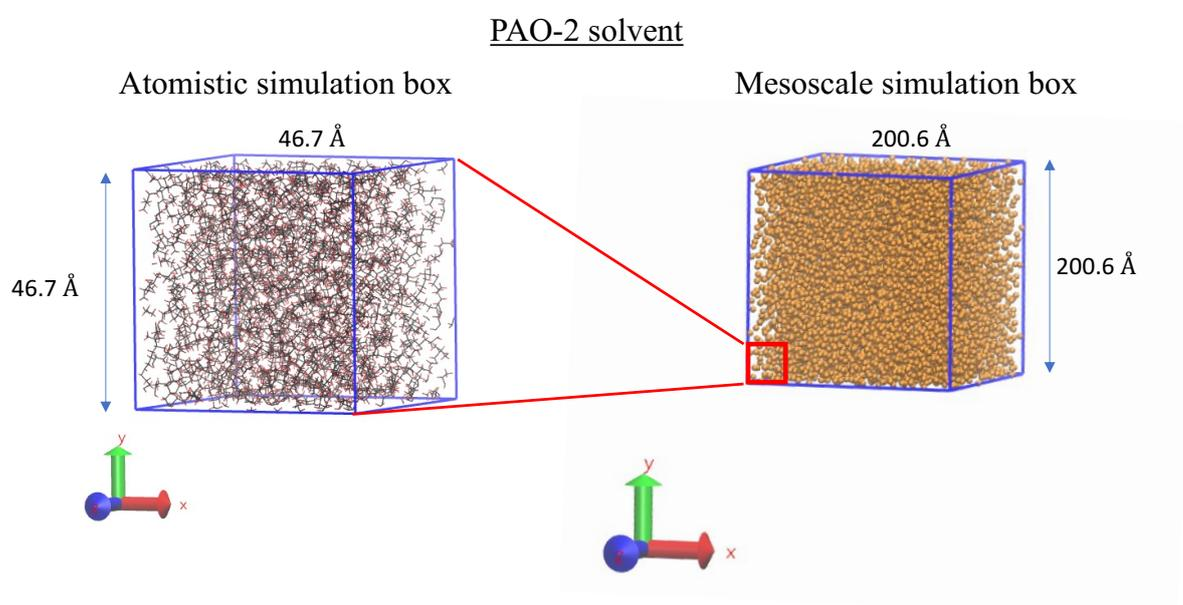
**Figure 3.2:** Representative simulation boxes of PAO-2 solvent in the atomistic scale consisting of 170 molecules and in the mesoscale consisting of 10980 molecules at 313 K.
