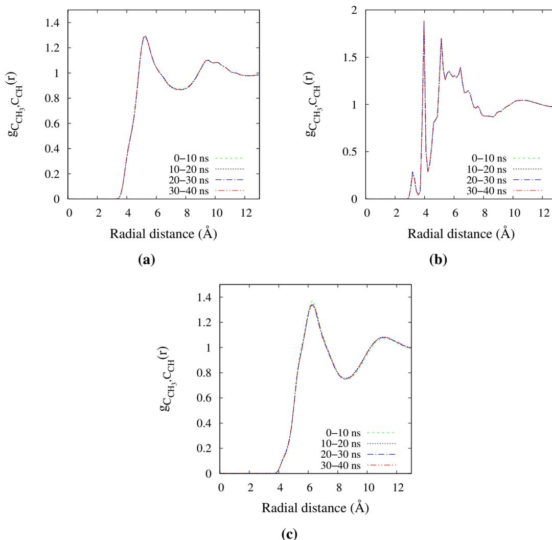
**Figure A1:** The radial distribution functions  $g_{o,p}(r)$  of (a)  $C_{CH_3}$ - $C_{CH_3}$  pair (b)  $C_{CH_3}$ - $C_{CH_2}$  pair and (c)  $C_{CH_3}$ - $C_{CH}$  pair in the solvent system computed from the data in the consequent windows of 10 ns during the production run of a simulation at 293 K. The overlapping radial distribution functions show that the system is well equilibrated.
