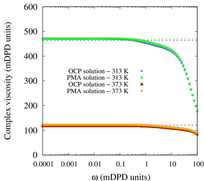
**Figure B8:** Complex viscosity ( $\eta^*(\omega)$ ) as a function of  $\omega$  for the OCP and PMA polymer solutions at 313 K and 373 K. The values agree with the  $\eta_0$  from Green-Kubo equation [188].
