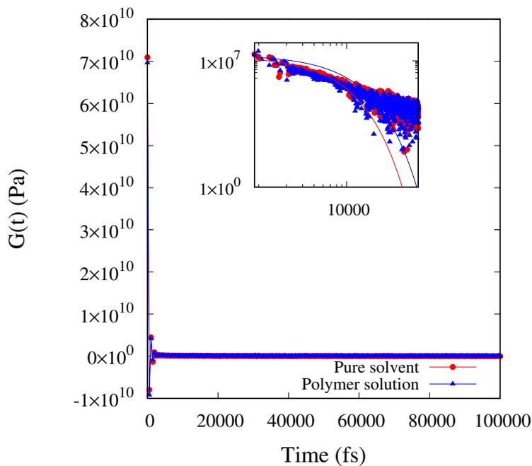
**Figure A6:**  $G(t)$  as a function of simulation time for pure solvent and polymer solution systems at 313 K. Inset shows  $G(t)$  values (points) smoothed by doing a running average between  $0.9t$  and  $1.1t$  as described by Sen et al. [200], and their corresponding fits (lines) of Equation 2.13 in Chapter 2.
