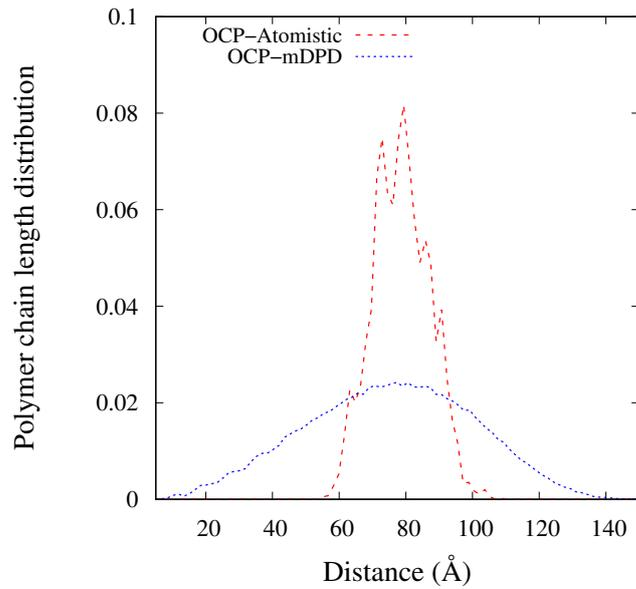
**Figure B4:** Polymer chain length distribution for OCP at 313 K in atomistic MD and mDPD.
