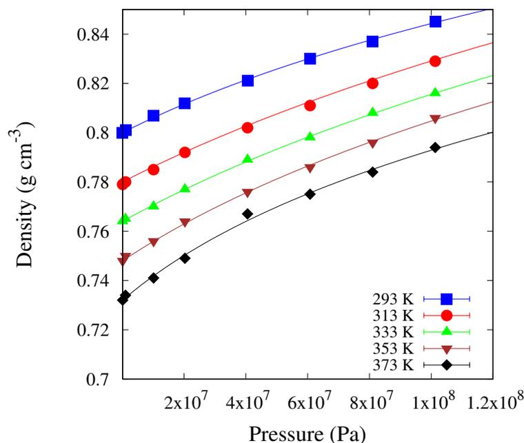
**Figure A2:** The density ( $\rho$ ) of pure solvent (PAO-2) as a function of pressure at different temperatures. The points show the simulated data, and the lines show the modified Tait equation fit as described in Equation 2.2 in Chapter 2.
