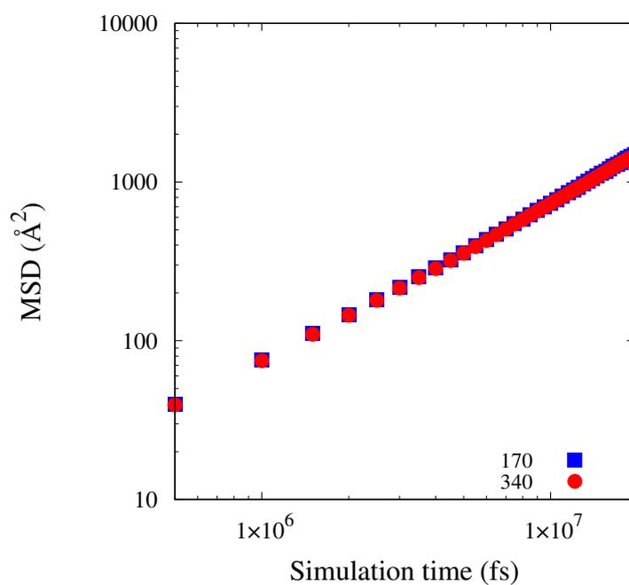
**Figure A5:** MSD of the PAO-2 molecules in pure solvent as a function of simulation time for a single simulation run at 313 K using multiple time origins. The closed symbols show the simulated values - blue (170 molecules) and red (340 molecules). The computed MSD shows that it is independent of the system size and the trajectories evolve similarly over time.
