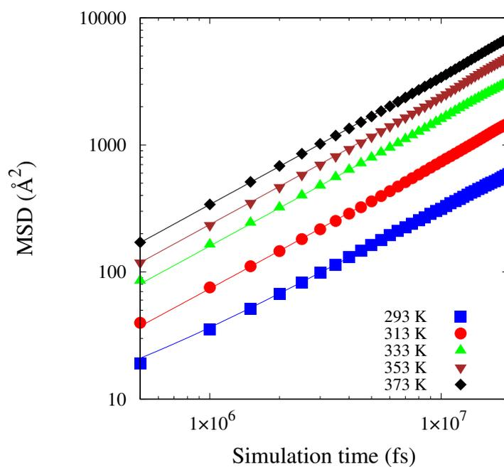
**Figure A4:** Mean squared displacement (MSD) of the PAO-2 molecules in pure solvent system as a function of simulation time for a single simulation run at different temperatures using multiple time origins. The closed symbols show the simulated MSD values. The lines show the fits of linear functions whose slope is used to compute the centre of mass self-diffusion coefficient,  $D_{\text{COM}}$ .
