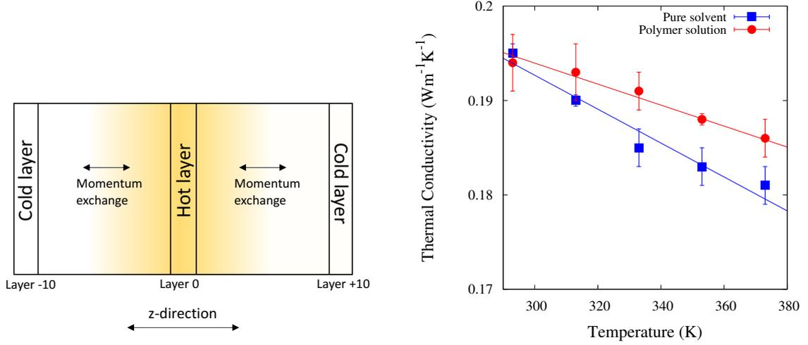
**Figure 2.9:** (Left) The schematic of reverse-NEMD applied in case of the present simulation study. (Right) The thermal conductivity ( $k$ ) of the pure solvent and polymer solution as a function of temperature. The closed symbols show the simulated data and the lines show the linear function fits as described in Equation 2.21.
