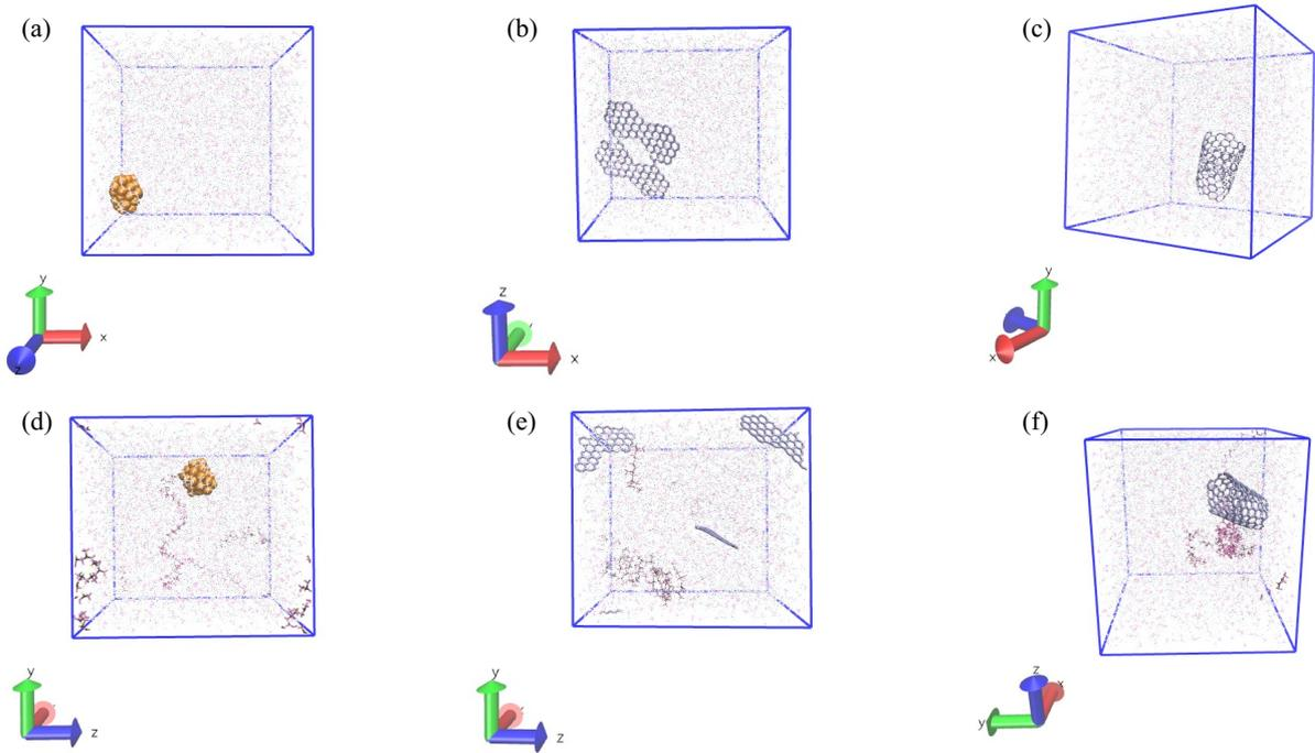
**Figure 4.2:** Simulation box of nanofluids (a) CU1, (b) GR1, (c) CN1, (d) CU2, (e) GR2, (f) CN2 at the end of the NPT equilibration run at 313 K. The orange coloured atoms represent Cu in (a) and (d). The purple coloured atoms represent 2D graphene in (b) and (e), and CNT in (c) and (f). The pink atoms represent OCP polymer chain in (d), (e) and (f). The translucent atoms represent PAO-2 solvent in all the simulation boxes.
