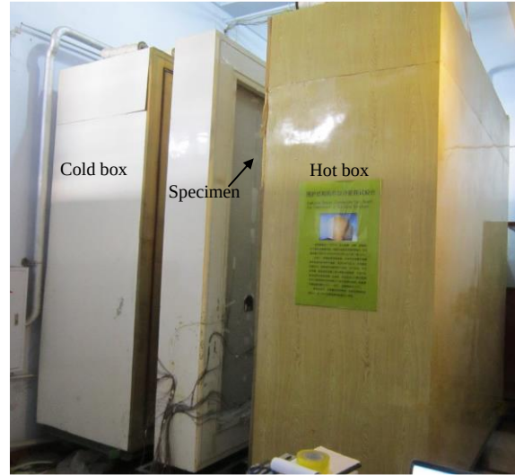
Fig. 5. A calibrated hot box system.
