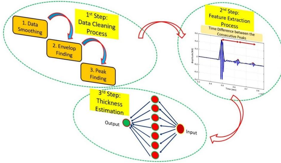
Figure 13. Workflow diagram of the thickness prediction process.
