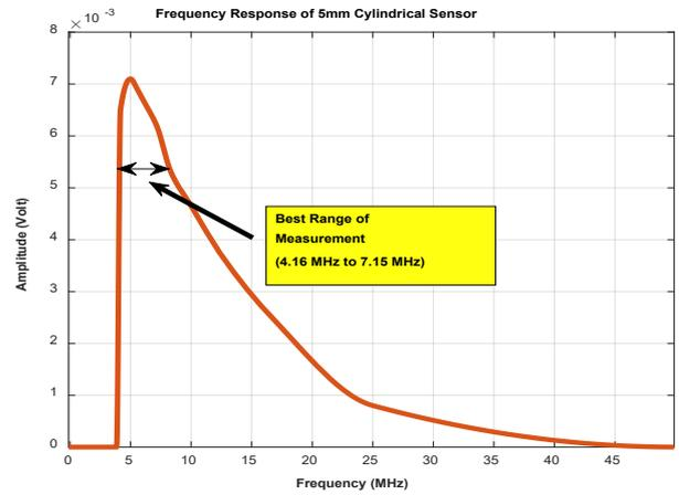
Figure 5. Frequency response of the 5 mm sensor.
