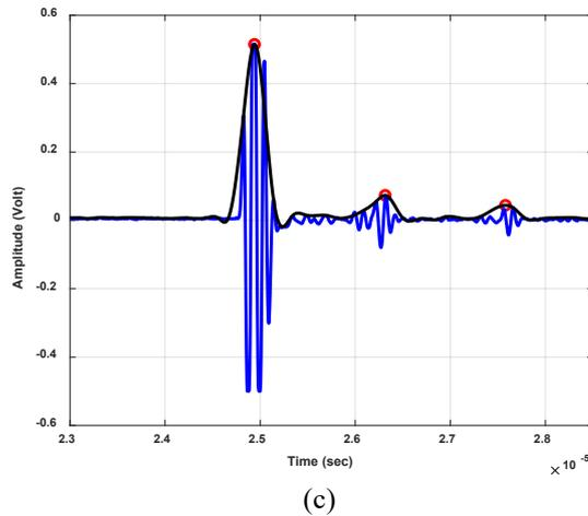
Figure 17. Time difference between the consecutive peaks shown by red dot and hole with a certain distance from top of the sample, (a) 1.6 mm; (b) 2.2 mm; (c) 3.9 mm.
