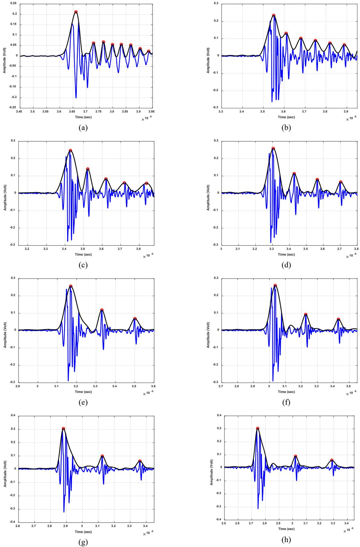
Figure 12. Time difference between the consecutive peaks shown by red dot, (a) 1 mm; (b) 2 mm; (c) 3 mm; (d) 4 mm; (e) 5 mm; (f) 6 mm; (g) 7 mm; (h) 8 mm.
