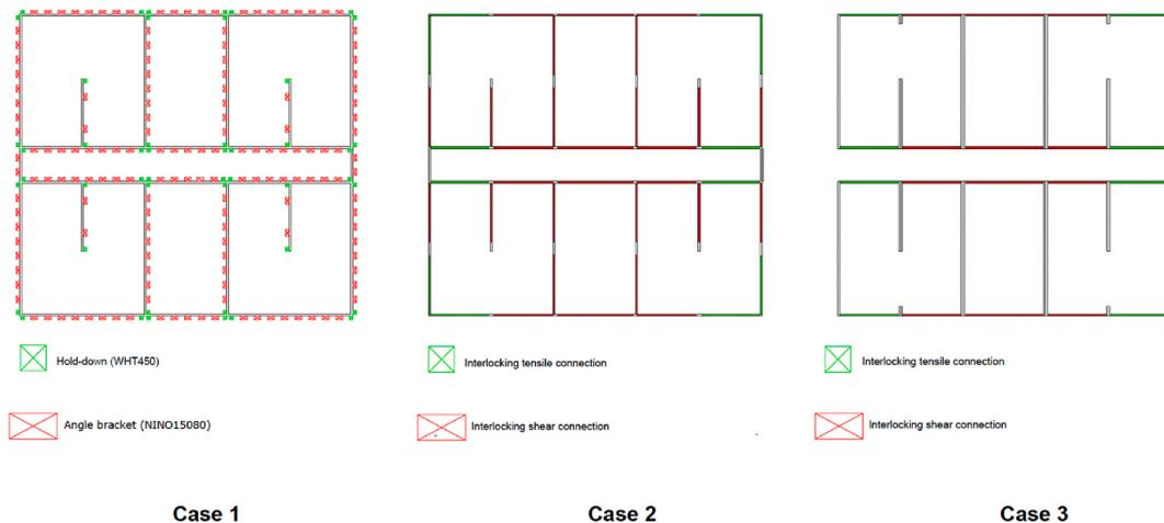
Fig. 18. Interlocking connection locations in different buildings.
