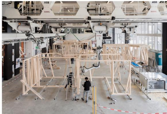
Fig. 11. The assembly of the DFABHOUSE [46].
