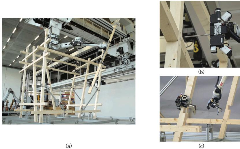
Fig. 12. Construction of CantiBox: (a) timber units during construction with the robotic arm; (b) robotic screwdriver on key components; (c) interlocking connections in the structures assembled by the robotic arm [48].
