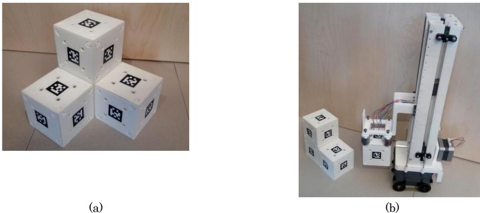
14 Figure 10. Prototypes of (a) the stigmergic building block and (b) the mobile robot [45]
