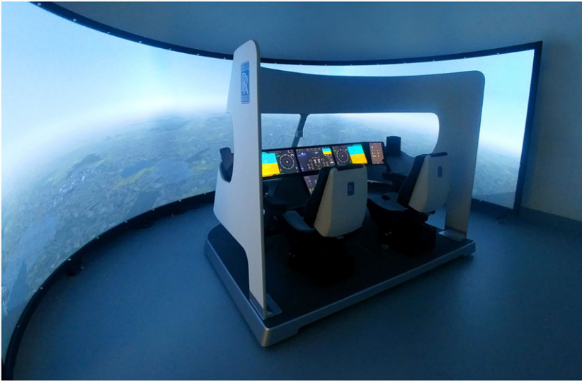
Figure 1. Future Systems Simulator in a working implementation of a conventional multi-crew configuration setup.
