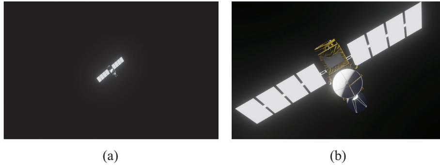
Fig. 4. Examples of synthetic data generated from Blender. (a) image captured at a camera position of (0, 0, 60 m). (b) image captured at a camera position of (0, 0, 10 m). Random rotation is applied to the target spacecraft.
