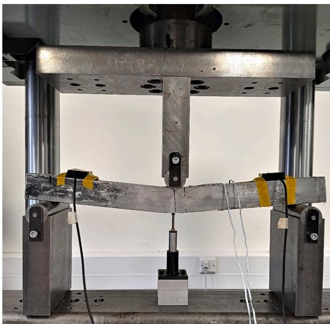
Fig. 8. Typical three-point bending test set-up.
