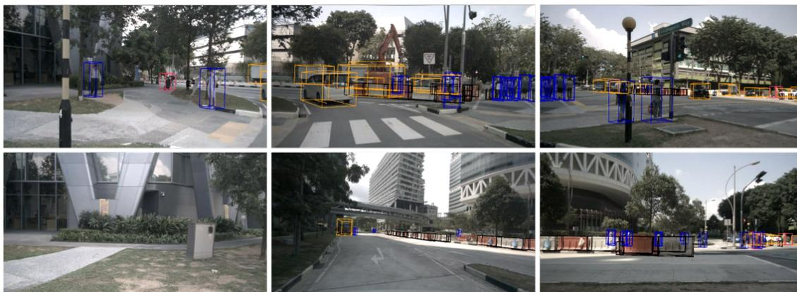
Figure 2.10 The sample annotations of 3D object detection in nuScenes [54] from the six cameras at one frame.
