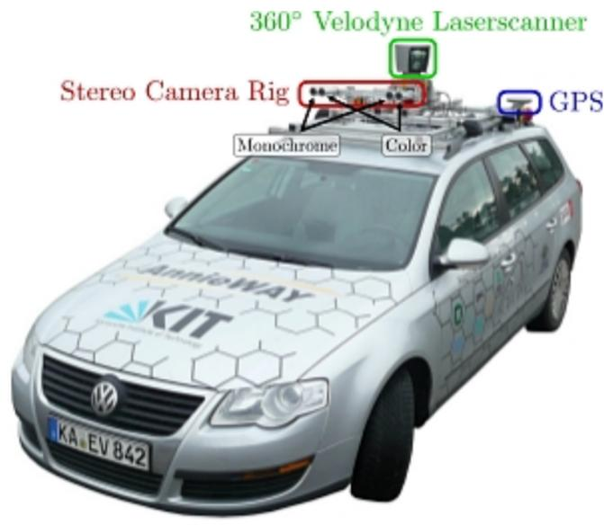
Figure 2.6 The sensor setup of KITTI [52] dataset. It contains a stereo camera set facing the front, a LiDAR, and a GPS/IMU.
