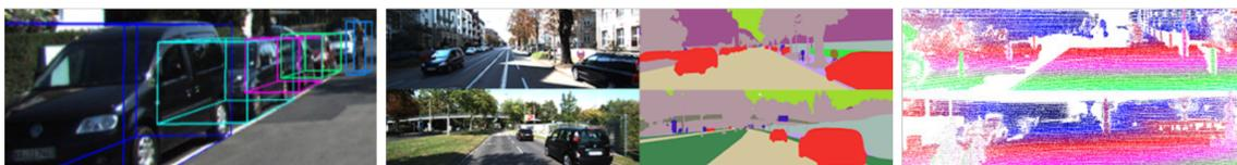
Figure 2.7 The sample data from KITTI [52] including labels of 3D object detection (left), semantic segmentation (centre), and depth prediction (right.)
