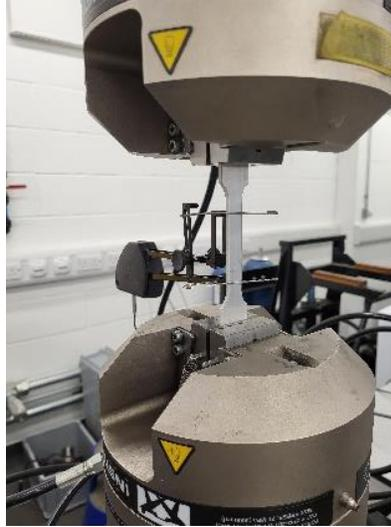
**Fig. 2.** Monotonic tensile test setup.
