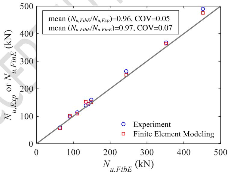
**Fig. 22.** Comparison between experimental and numerical compressive capacities.
