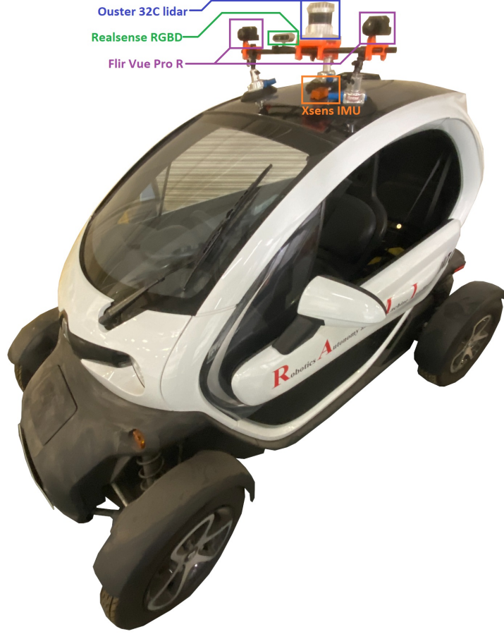
Figure 2.1: Figure of the capture vehicle - a Renault Twizy. The sensors utilised include; left and right thermal cameras, a 32 channel Lidar, and an active RGBD camera.
