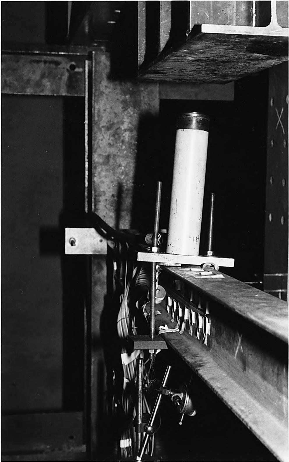
Fig. 6.18 Stiffeners For Beam B2 (See Fig. 6.3)
