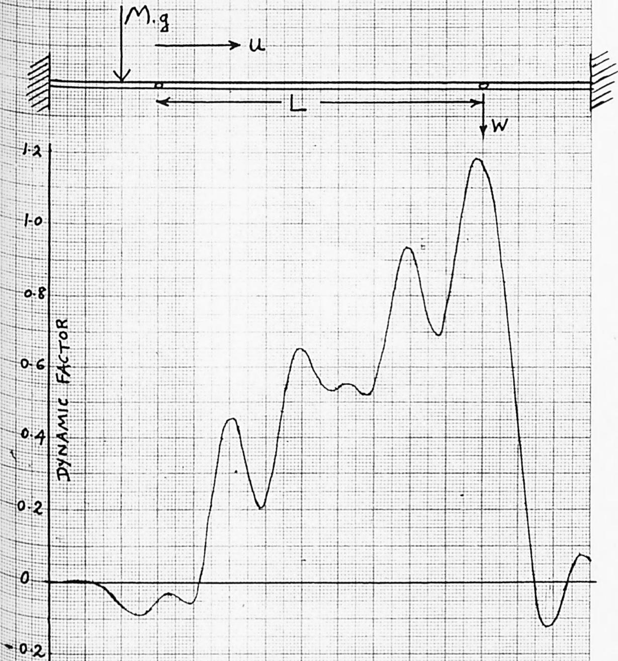
CANTILEVER DEFLECTION "W" DURING TRANSIT OF A SINGLE LOAD AT A SPEED CORRESPONDING TO  $\beta = 4$
