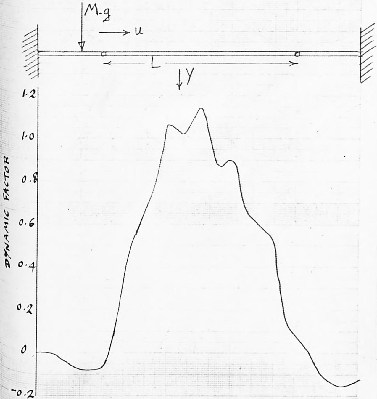
MIDSPAN DEFLECTION  $Y$  DURING TRANSIT OF A SINGLE LOAD
