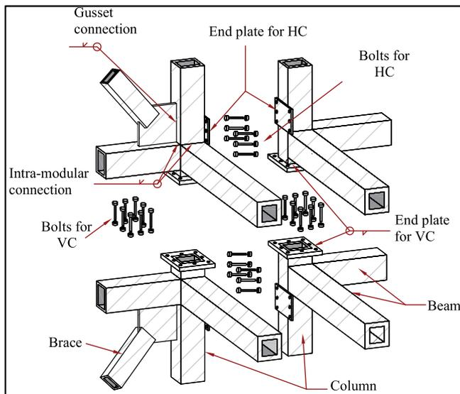
**Fig. 5.** Vertical and horizontal IMC details [56].
