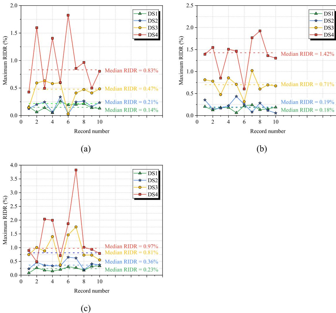
Fig. 13. The maximum residual inter-story drift ratio of (a) 4-story (b) 8-story (c) 12-story modular steel buildings subjected to mainshocks scaled at four IDR-based damage states.
