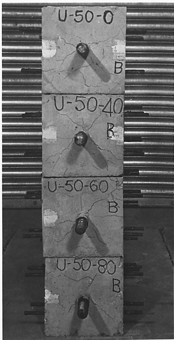
FIG. 6.18 TYPICAL FAILURE MODES UNDER TENSION RELEASE - HYBAR
