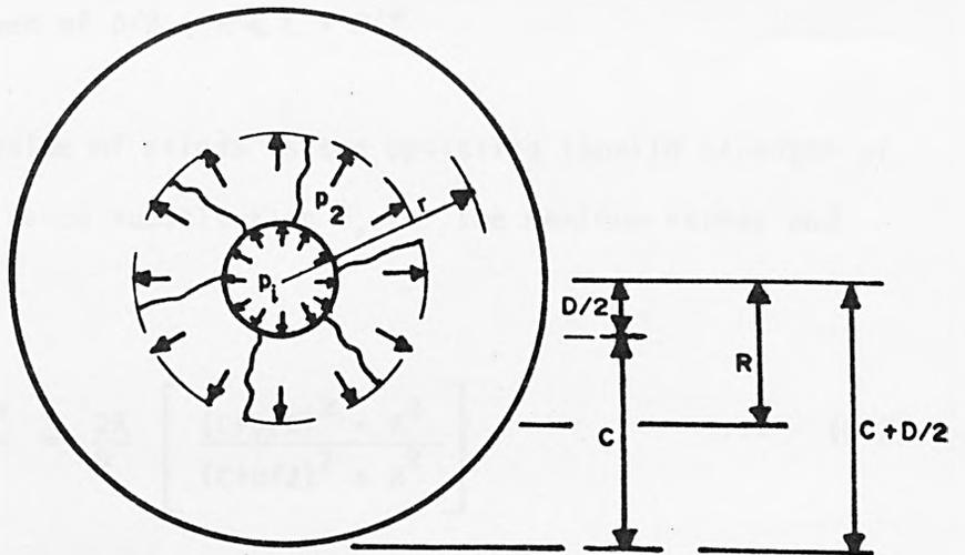
FIG. 5.4 INTERNAL CRACKING SURROUNDING REINFORCEMENT BAR
