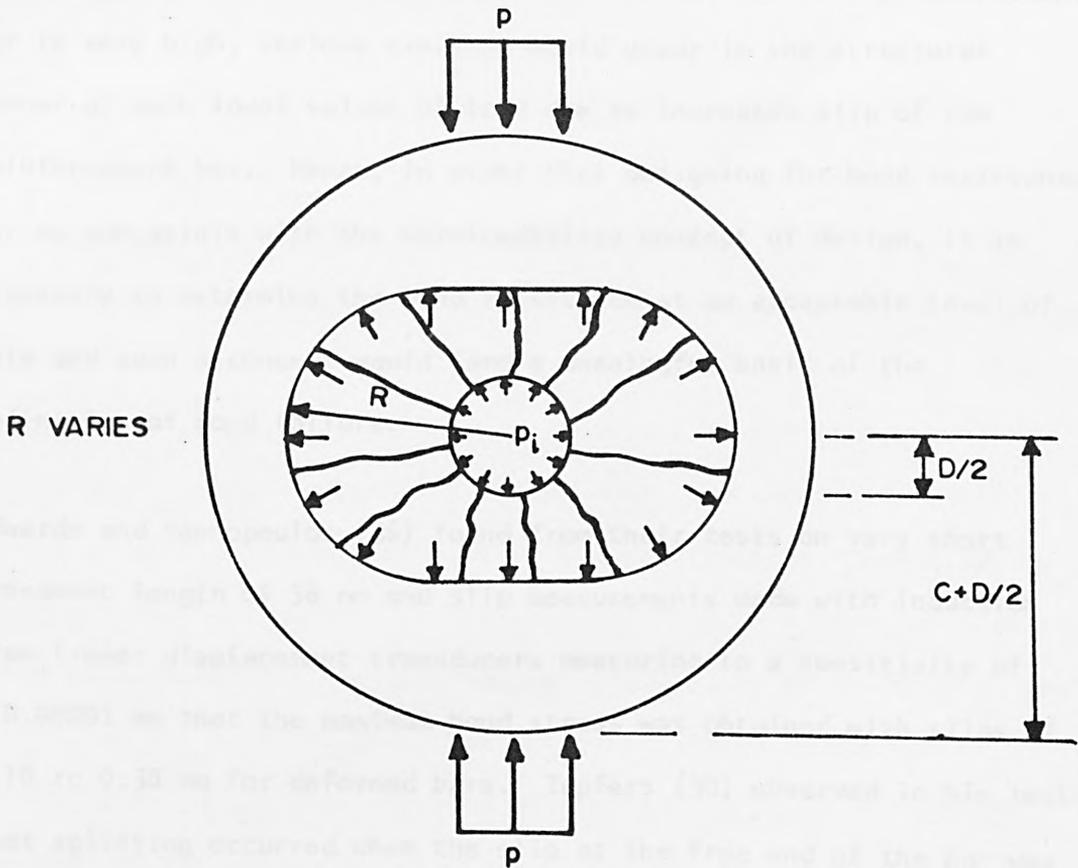
FIG. 5.8 INTERNAL CRACKING IN CONCRETE RING UNDER UNIDIRECTIONAL PRESSURE
