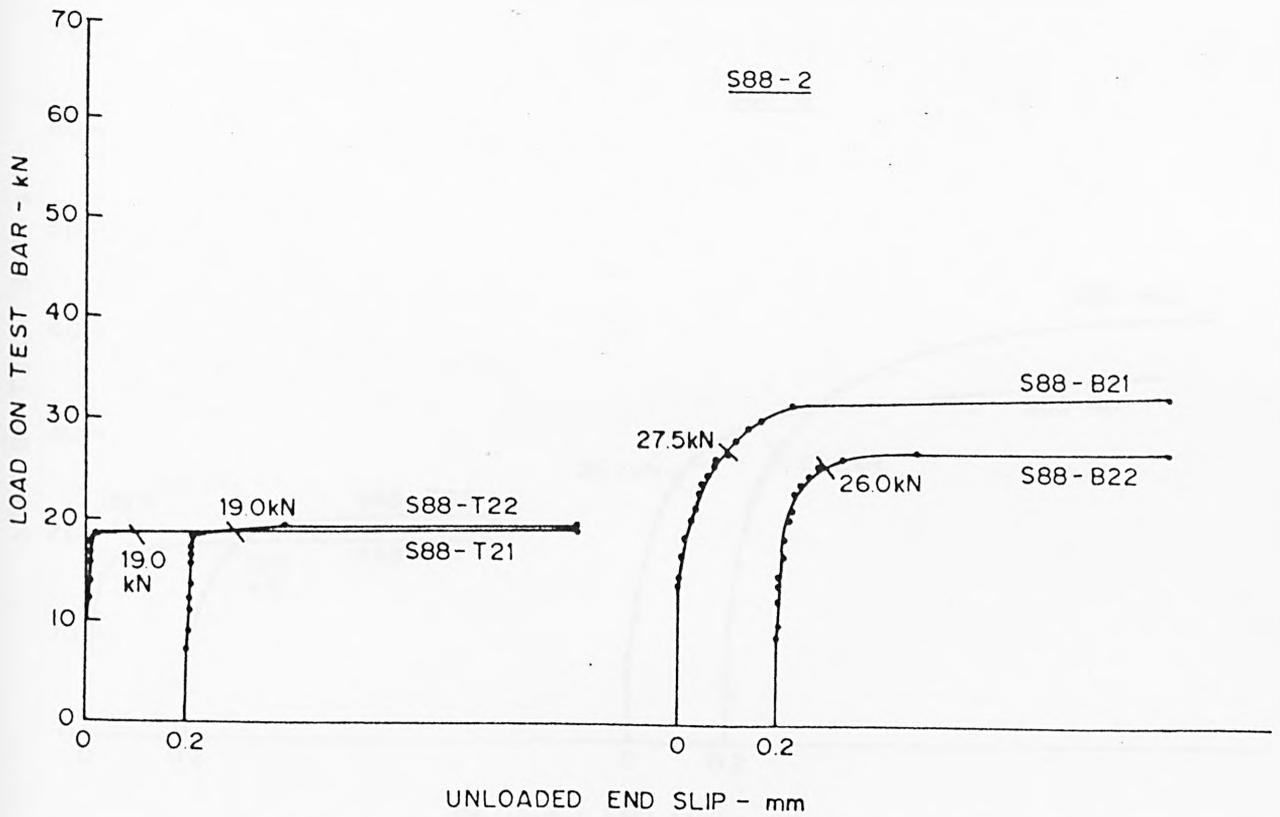
FIG A 25 LOAD-SLIP CHARACTERISTICS AT UNLOADED END - SQUARE-TWISTED BAR
