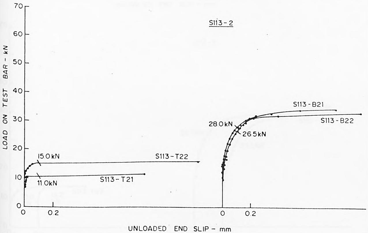
FIG A23 LOAD-SLIP CHARACTERISTICS AT UNLOADED END - SQUARE-TWISTED BAR
