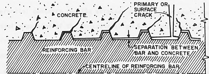
FIG. 5.10 SECTION THROUGH REINFORCING BAR AND CONCRETE
