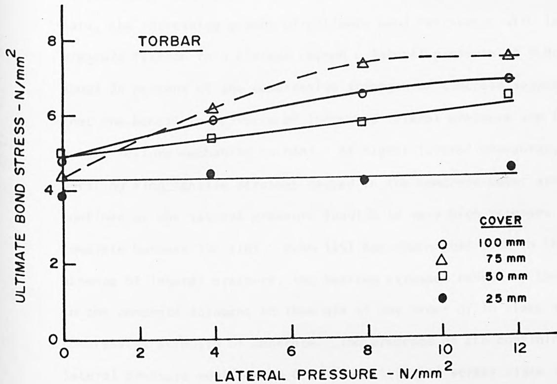
FIG. 7.4 VARIATION OF ULTIMATE BOND STRESS WITH LATERAL PRESSURE - TORBAR
