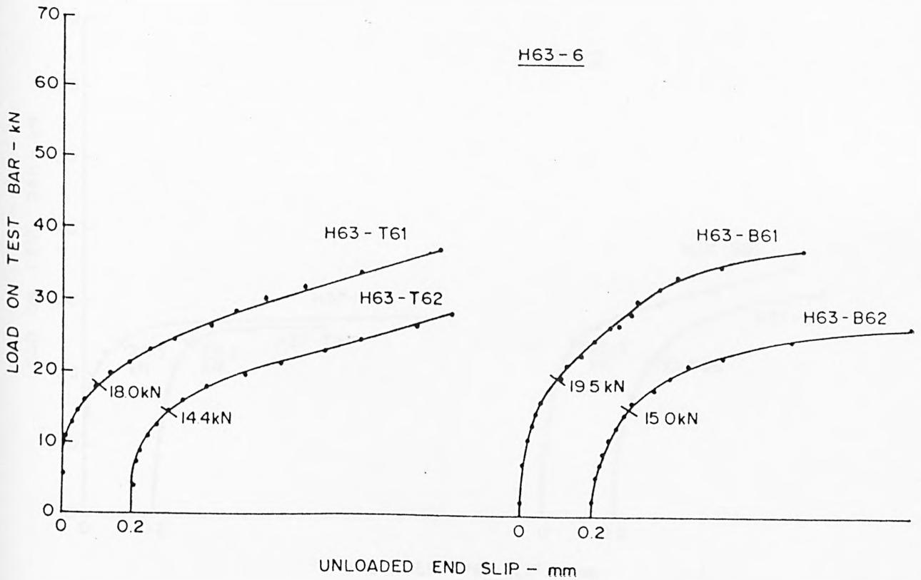
FIG A 20 LOAD-SLIP CHARACTERISTICS AT UNLOADED END-HYBAR
