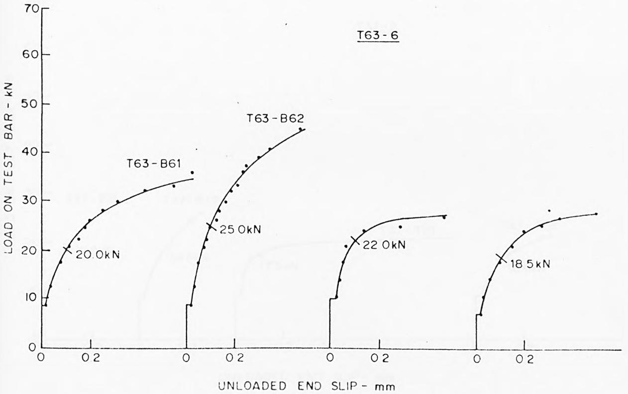
FIG A12 LOAD-SLIP CHARACTERISTICS AT UNLOADED END - TORBAR
