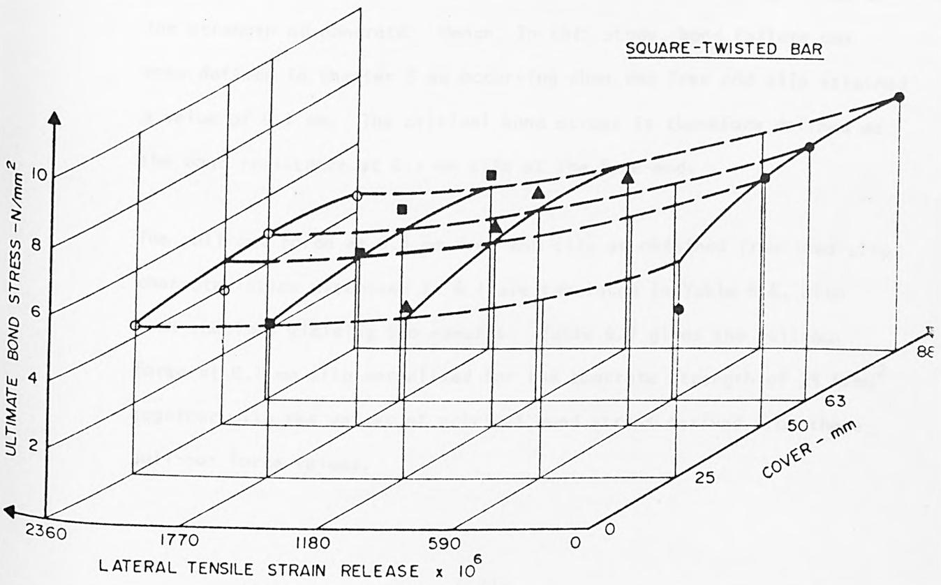
FIG. 6.6 VARIATION OF BOND STRESS WITH COVER AND TENSION RELEASE
