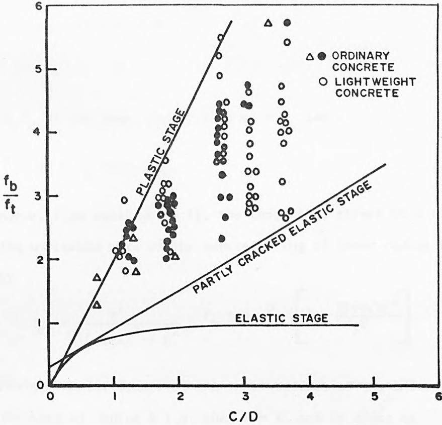
FIG. 5.3 EFFECT OF THICKNESS OF CONCRETE COVER UPON BOND CAPACITY (after Tefpers)
