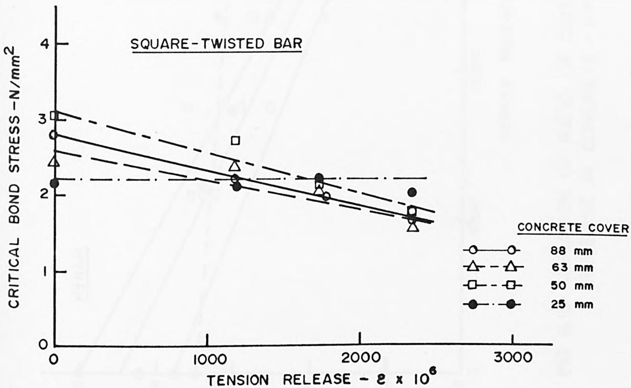
FIG. 6.12 VARIATION OF CRITICAL BOND STRESS WITH TENSION RELEASE - SQUARE-TWISTED BAR
