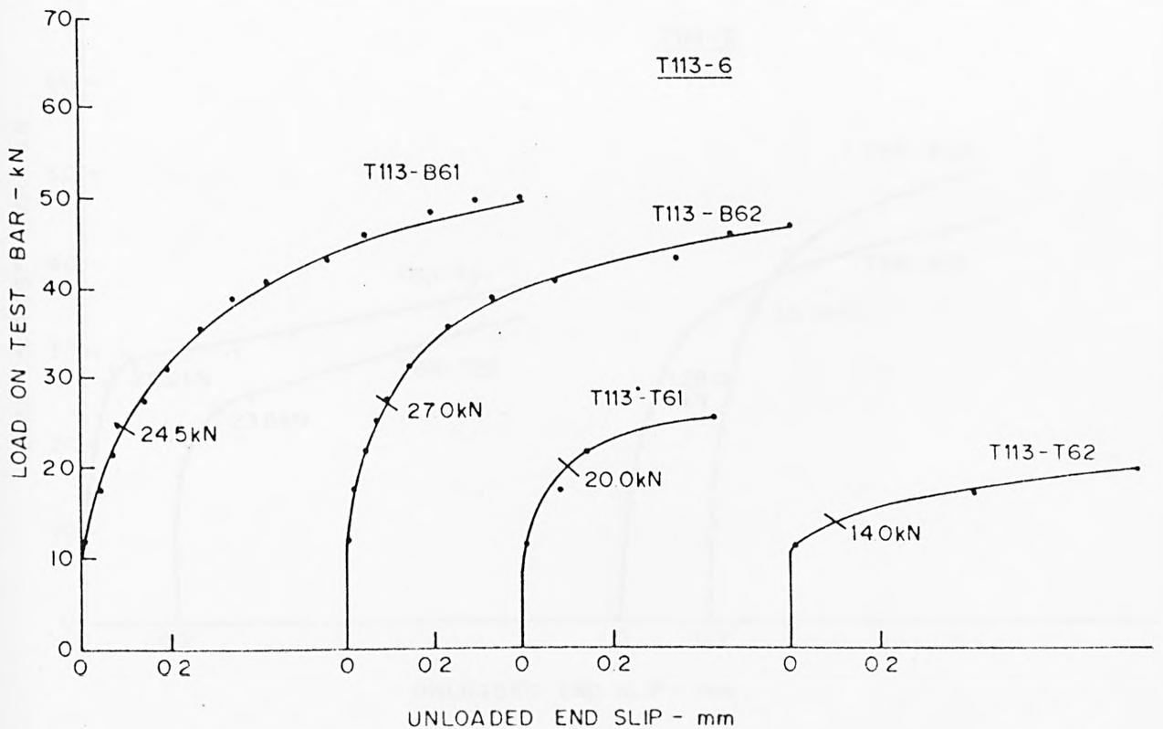
FIG A8 LOAD-SLIP CHARACTERISTICS AT UNLOADED END - TORBAR
