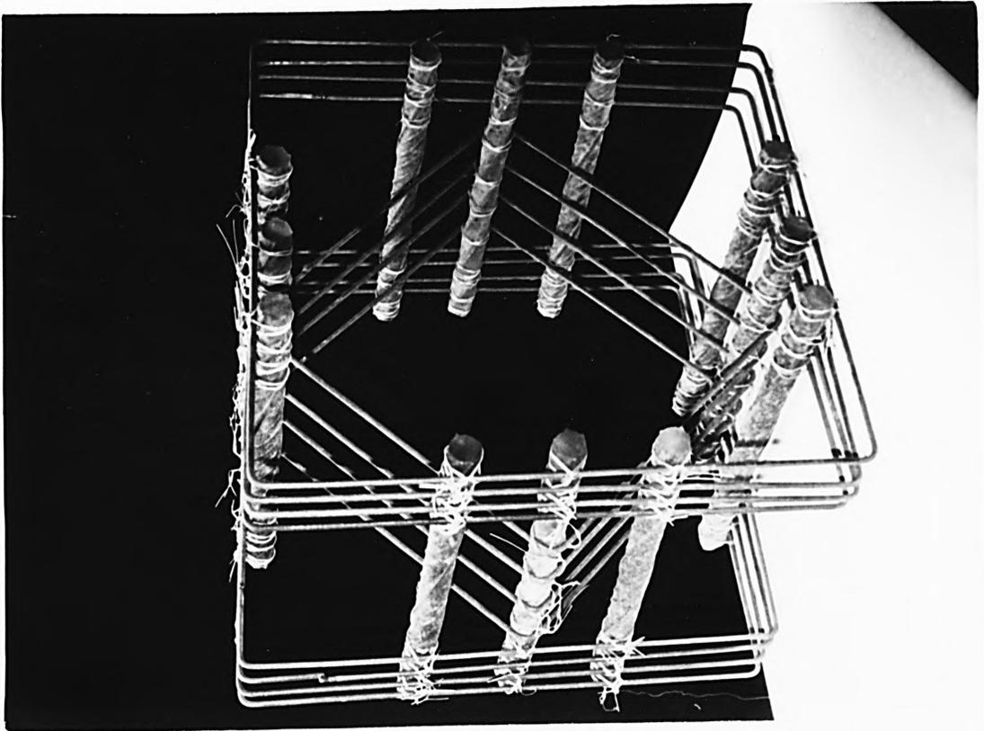
FIG. 4.2 ASSEMBLED SECONDARY REINFORCEMENT CAGE
