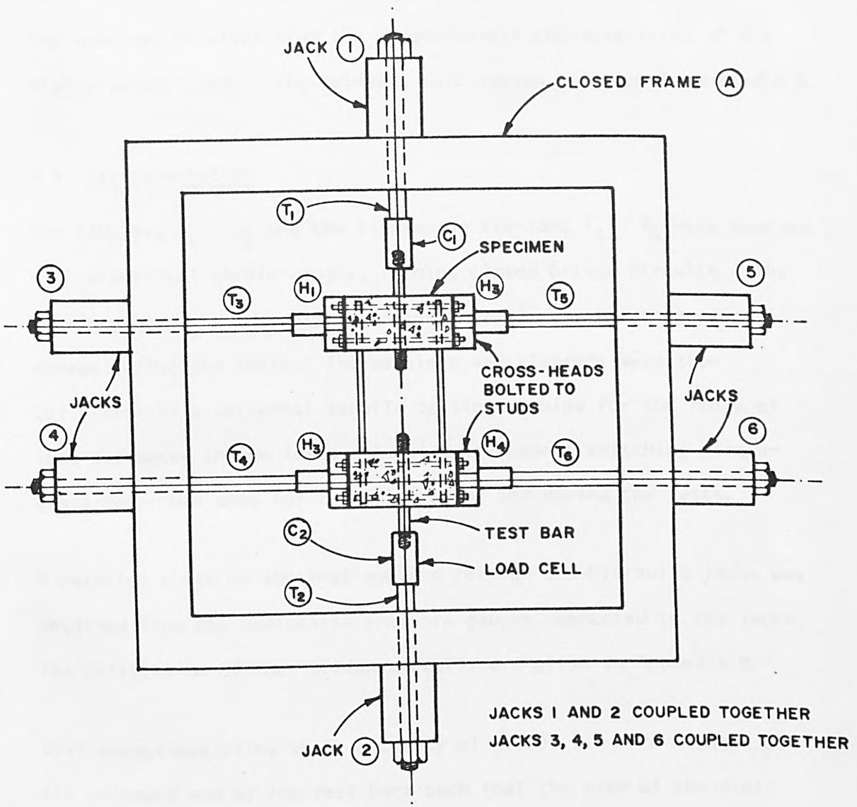
FIG. 3.5 SCHEMATIC DIAGRAM OF TEST ARRANGEMENT
