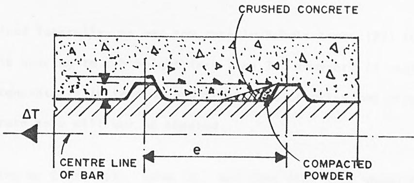
FIG. 5.1 BEARING OF RIB AGAINST CONCRETE
