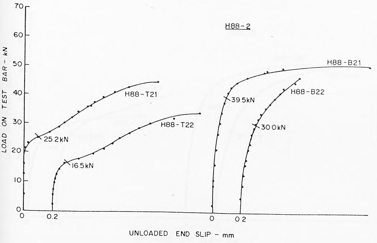
FIG A17 LOAD-SLIP CHARACTERISTICS AT UNLOADED END - HYBAR
