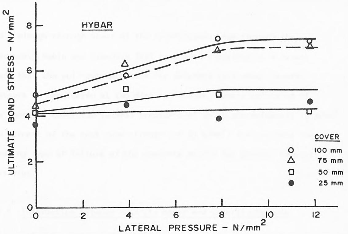
FIG. 7.5 VARIATION OF ULTIMATE BOND STRESS WITH LATERAL PRESSURE - HYBAR
