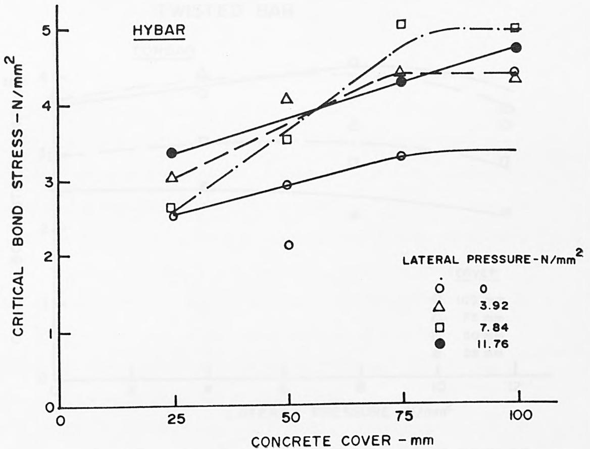
FIG. 7.11 VARIATION OF CRITICAL BOND STRESS WITH CONCRETE COVER - HYBAR
