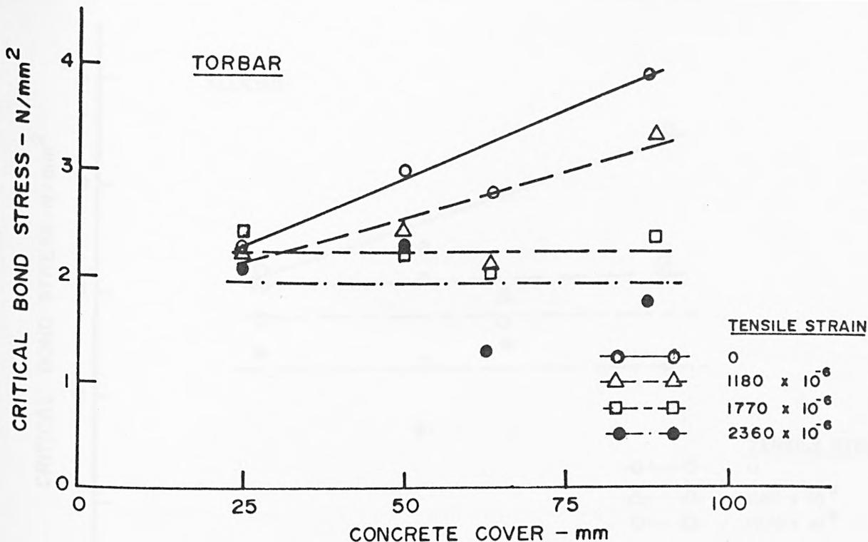
FIG. 6.7 VARIATION OF CRITICAL BOND STRESS WITH COVER - TORBAR
