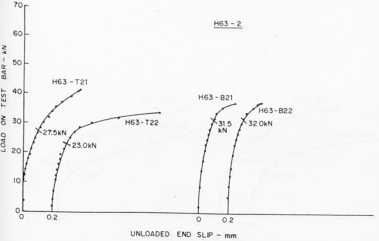
FIG. A19 LOAD-SLIP CHARACTERISTICS AT UNLOADED END - HYBAR
