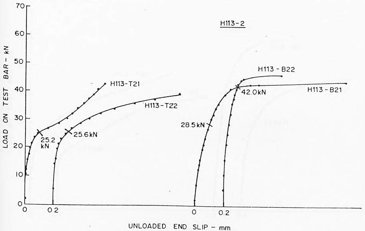
FIG. A15 LOAD-SLIP CHARACTERISTICS AT UNLOADED END - HYBAR
