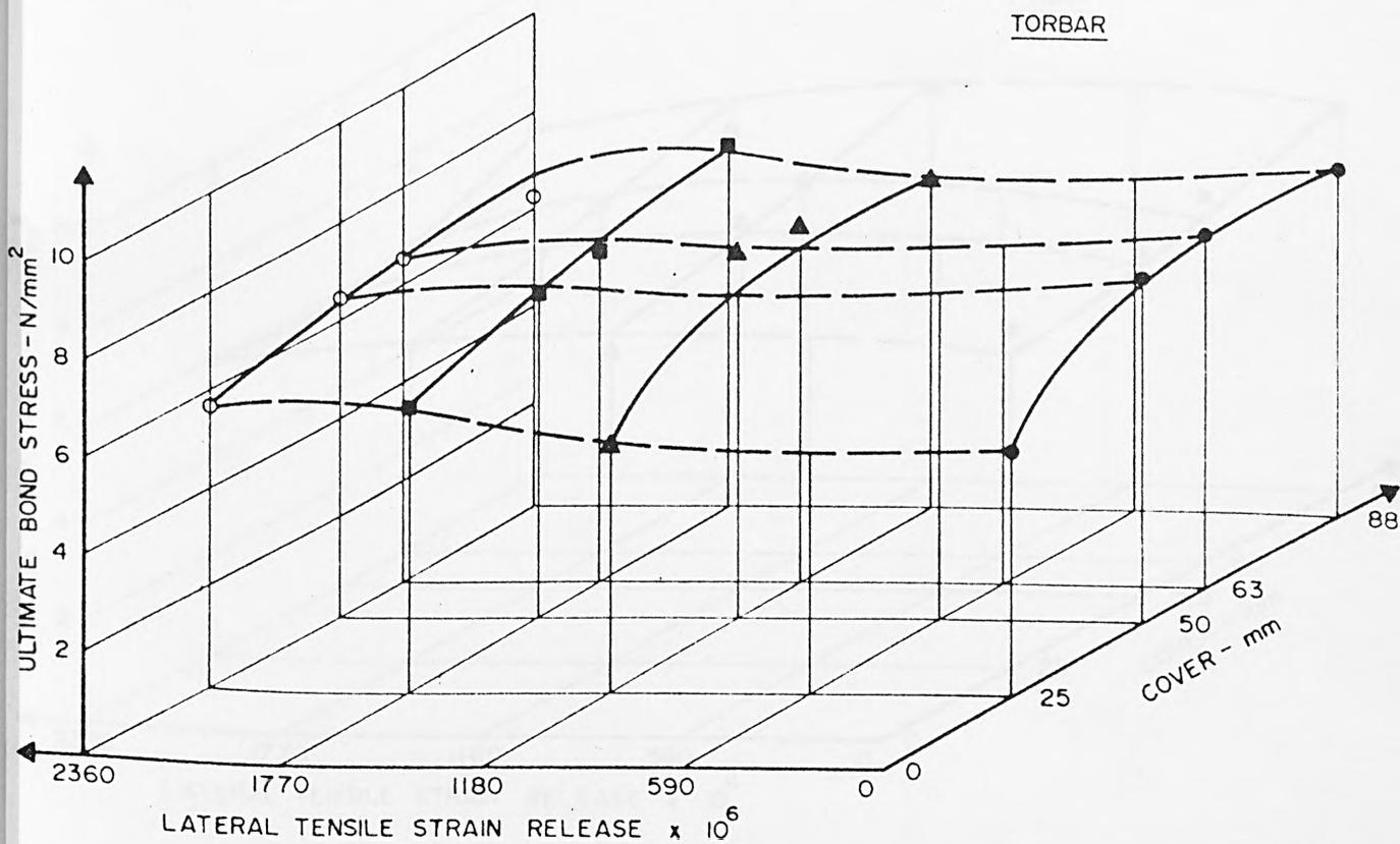
FIG 6.4 VARIATION OF BOND STRESS WITH COVER AND TENSION RELEASE
