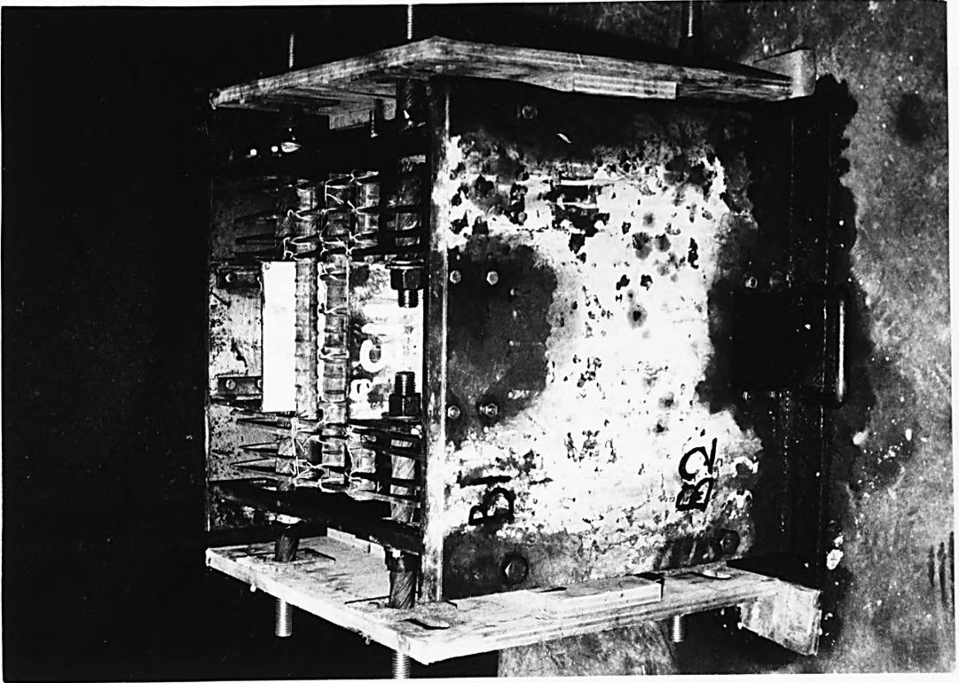
FIG. 4.4 SPECIMEN ASSEMBLY BEFORE CASTING
