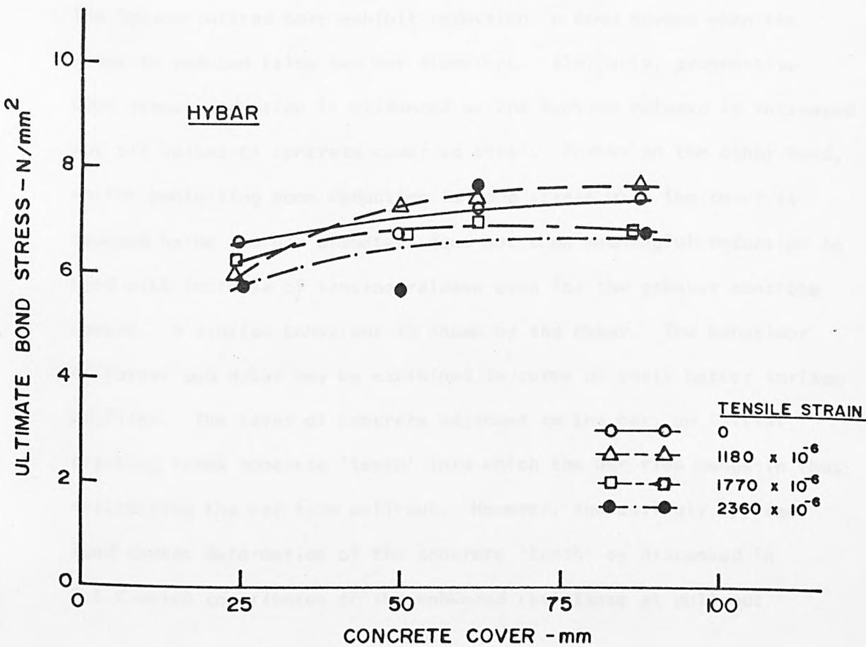
FIG. 6.3 VARIATION OF ULTIMATE BOND STRESS WITH COVER - HYBAR
