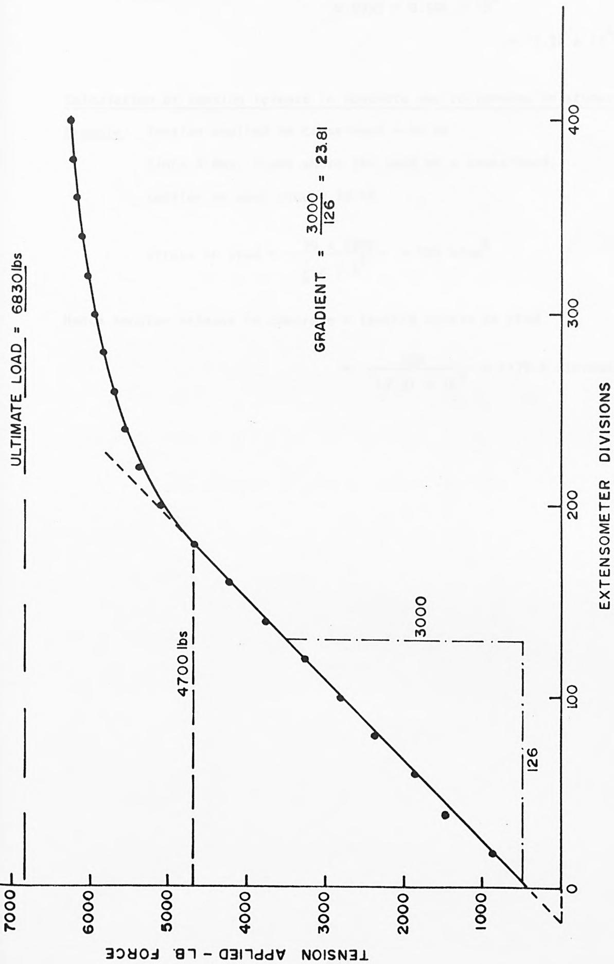
FIG. B.2 STRESS-STRAIN CHARACTERISTIC OF HIGH TENSILE STEEL STUD
