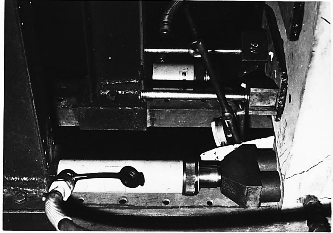
FIG. 4.8 JACKS APPLYING LATERAL PRESSURE
