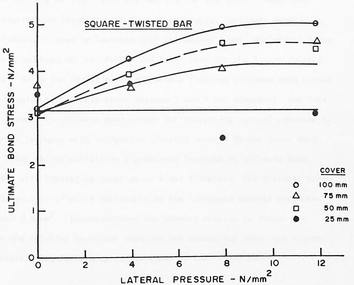
FIG. 7.6 VARIATION OF ULTIMATE BOND STRESS WITH LATERAL PRESSURE - SQUARE - TWISTED BAR
