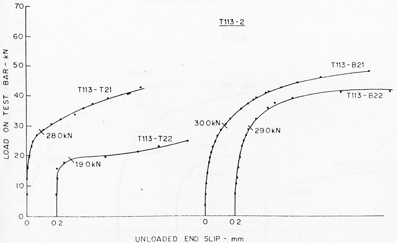
FIG A7 LOAD - SLIP CHARACTERISTICS AT UNLOADED END - TORBAR
