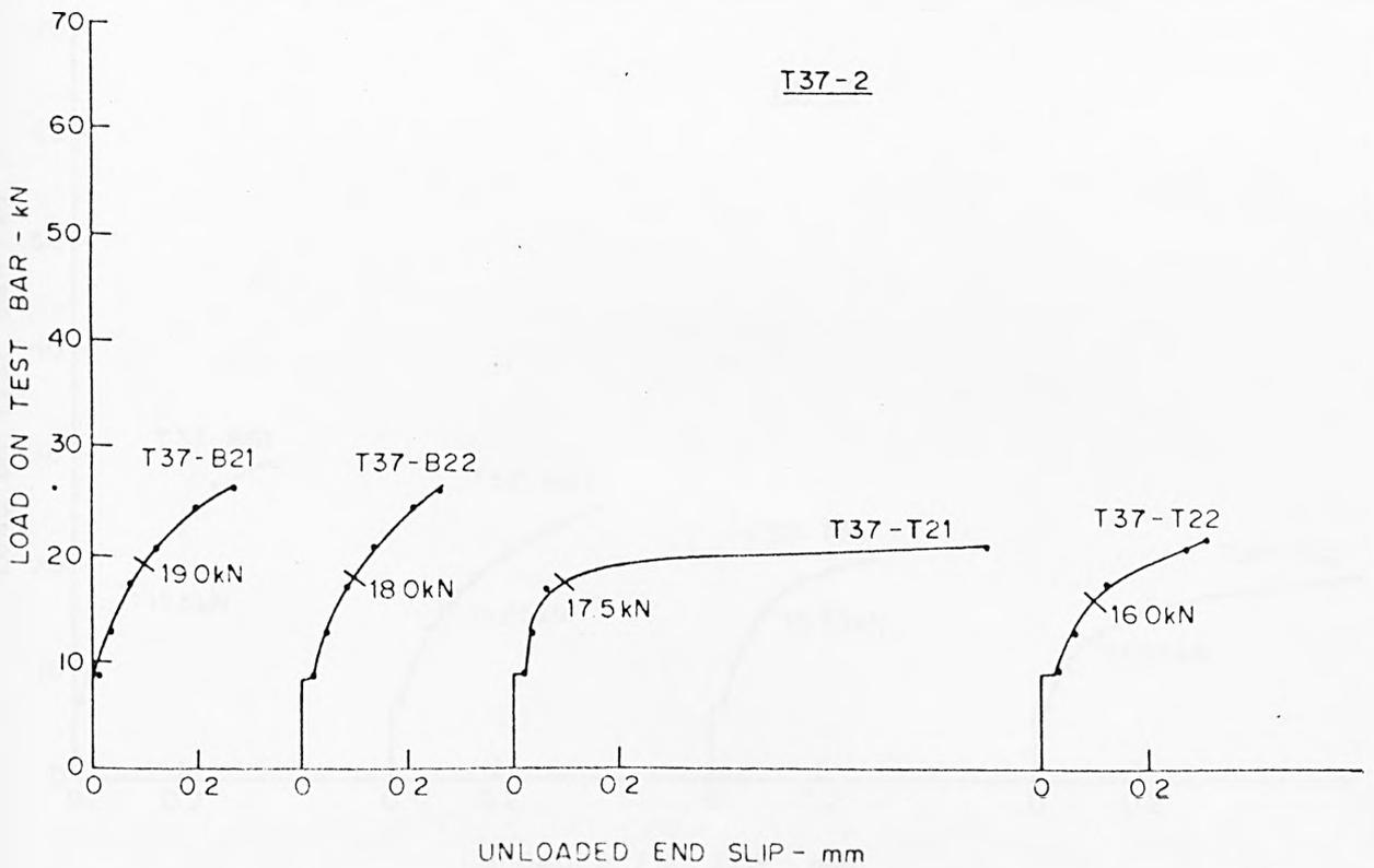
FIG A13 LOAD-SLIP CHARACTERISTICS AT UNLOADED END - TORBAR
