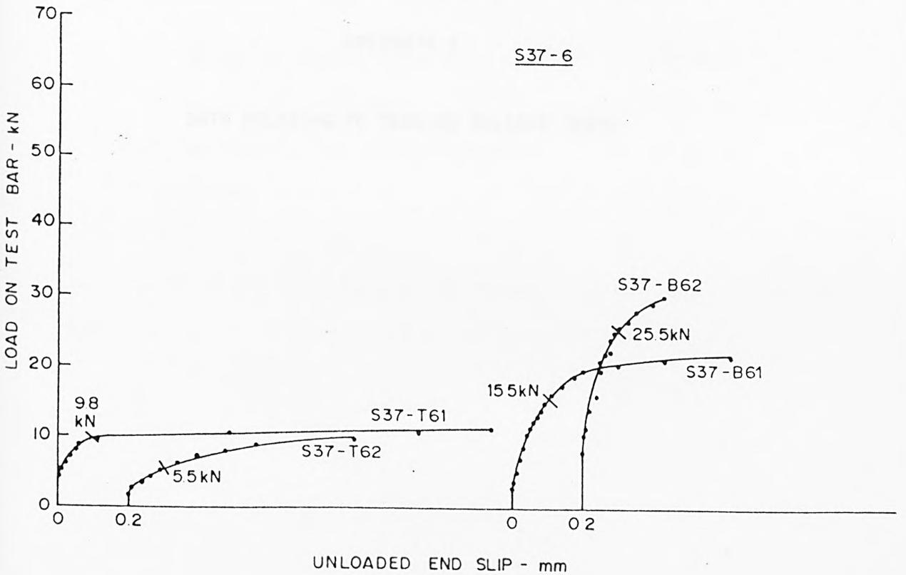
FIG A 30 LOAD-SLIP CHARACTERISTICS AT UNLOADED END - SQUARE-TWISTED BAR
