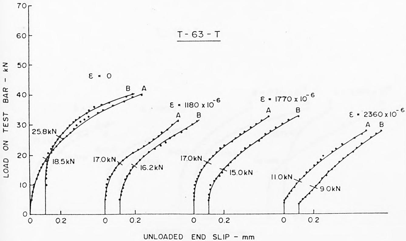
FIG. A.1 LOAD - SLIP CHARACTERISTICS AT UNLOADED END - TORBAR
