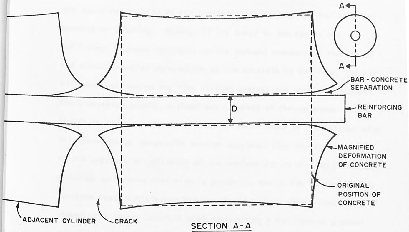
FIG. 5.11 MAGNIFIED DEFORMATION SHOWING SEPARATION BETWEEN CONCRETE AND BAR (After Lutz)
