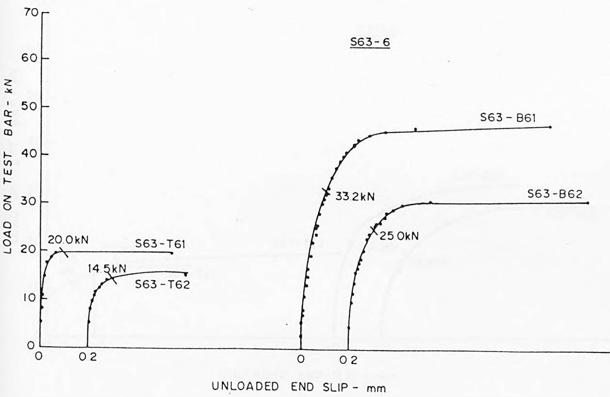
FIG A.28 LOAD-SLIP CHARACTERISTICS AT UNLOADED END - SQUARE-TWISTED BAR
