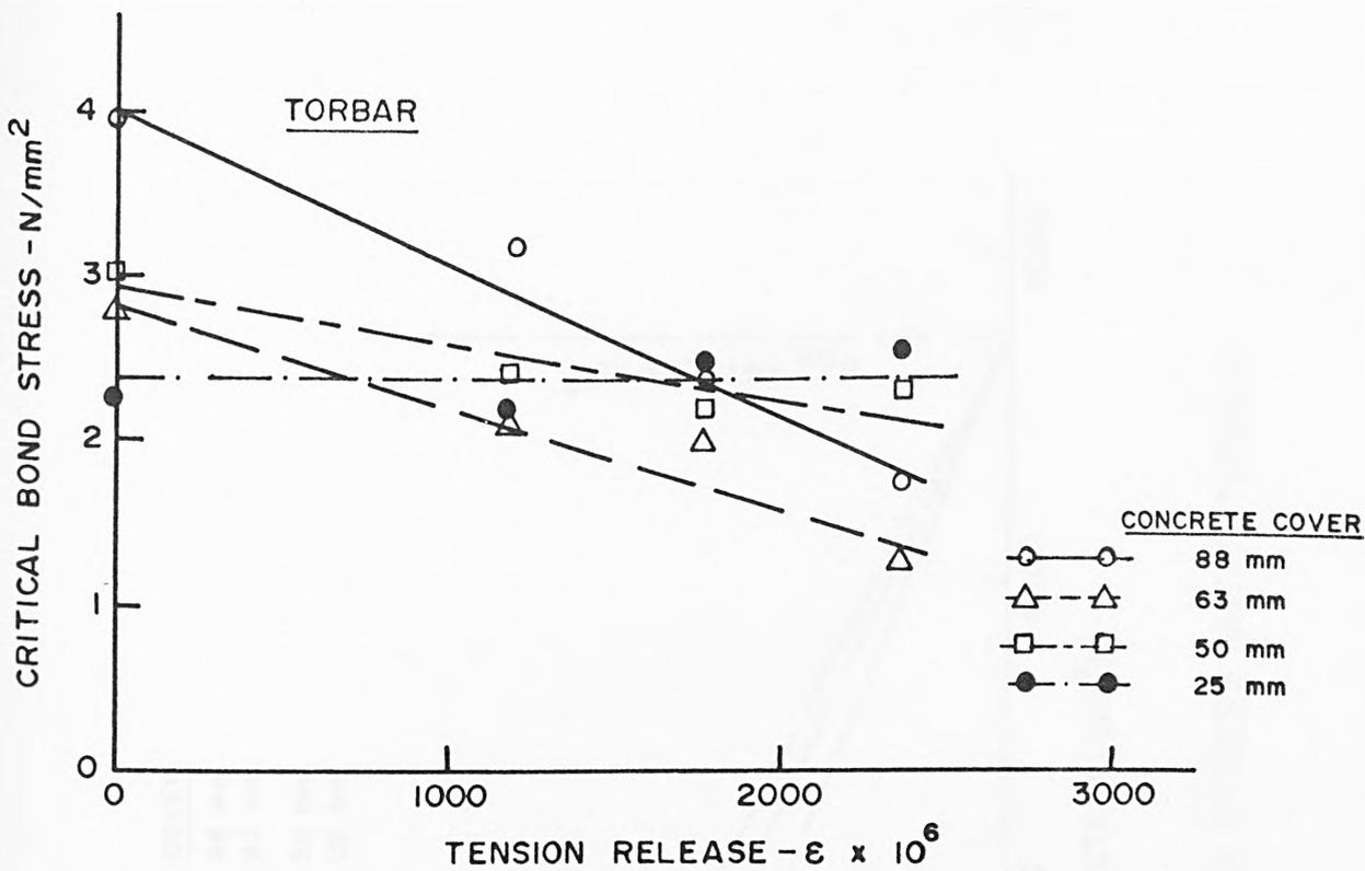
FIG. 6.11 VARIATION OF CRITICAL BOND STRESS WITH TENSION RELEASE - TORBAR
