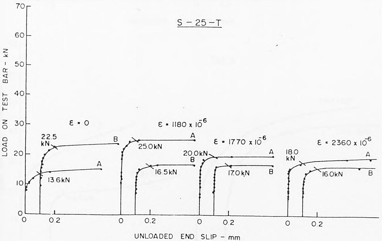
FIG A6 LOAD-SLIP CHARACTERISTICS AT UNLOADED END - SQUARE-TWISTED BAR
