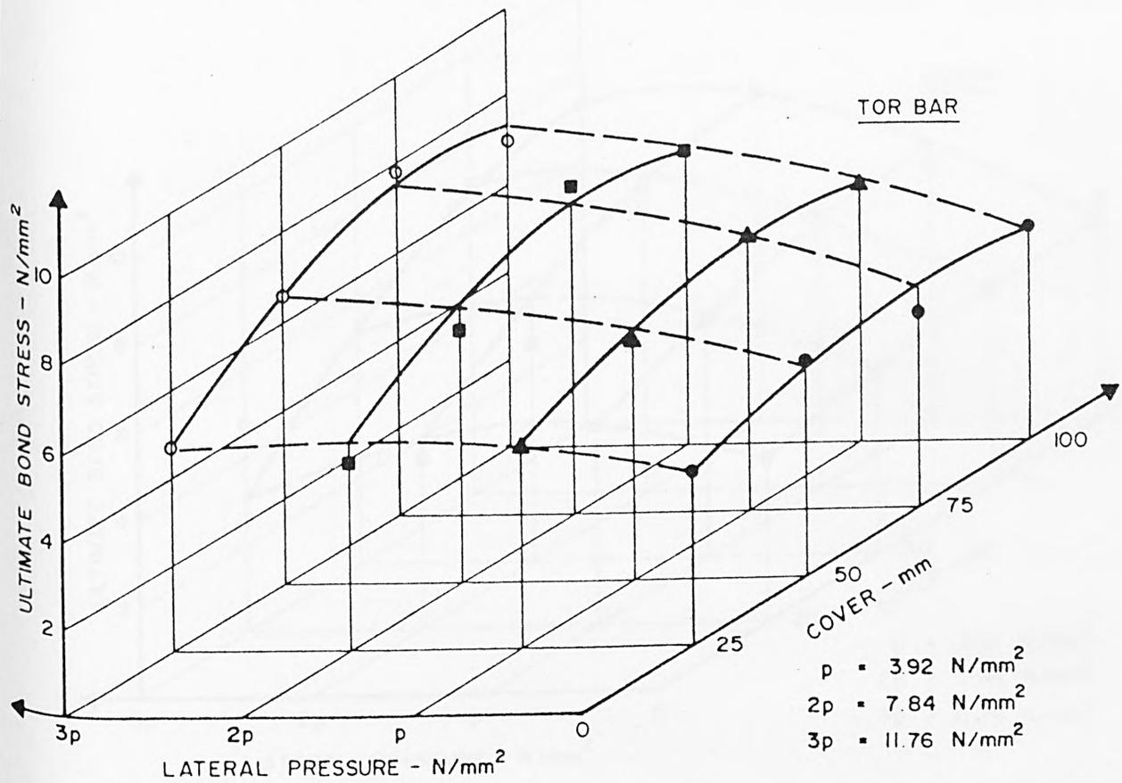
FIG. 7.7 VARIATION OF BOND STRESS WITH COVER AND LATERAL PRESSURE (Top) CRITICAL BOND STRESS, (Bottom) ULTIMATE BOND STRESS.
