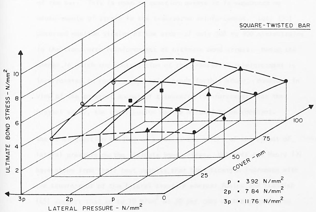
FIG 7.9 VARIATION OF BOND STRESS WITH COVER AND LATERAL PRESSURE (Top) CRITICAL BOND STRESS, (Bottom) ULTIMATE BOND STRESS
