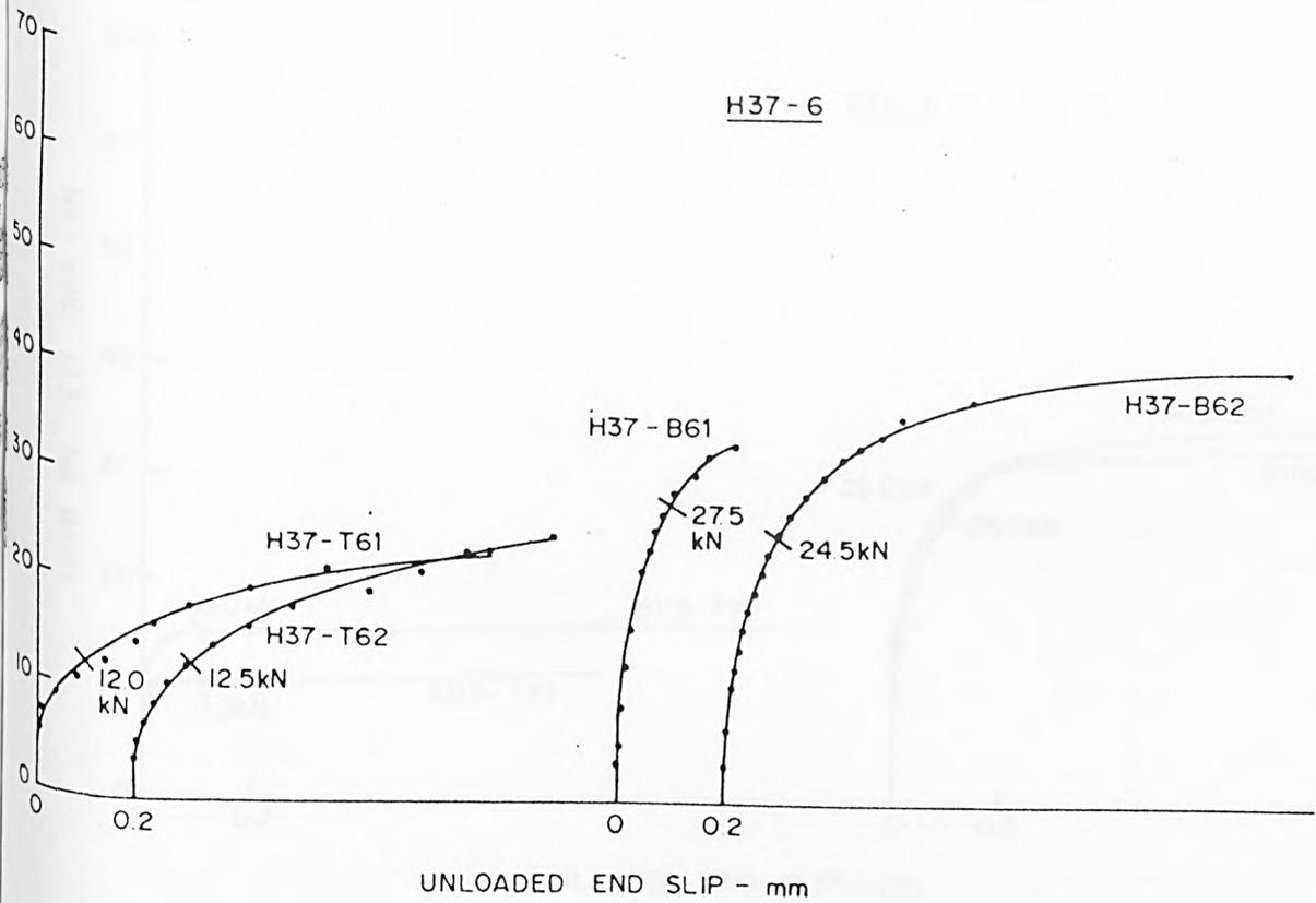
FIG A22 LOAD-SLIP CHARACTERISTICS AT UNLOADED END - HYBAR
