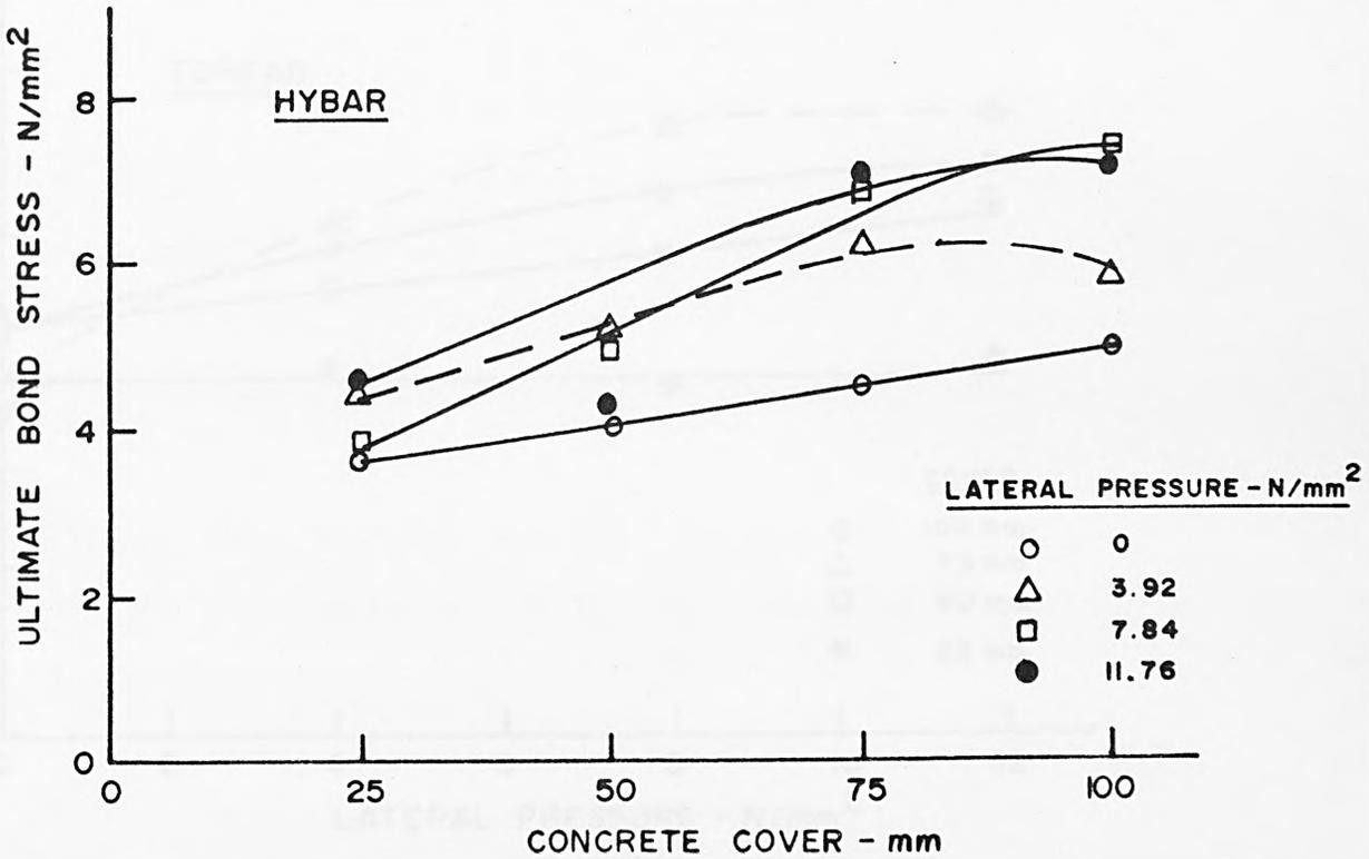
FIG. 7.2 VARIATION OF ULTIMATE BOND STRESS WITH CONCRETE COVER - HYBAR
