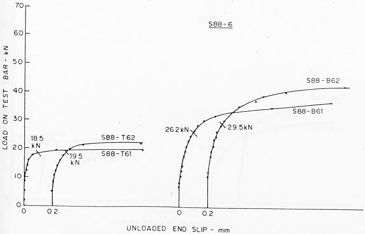
FIG A.26 LOAD-SLIP CHARACTERISTICS AT UNLOADED END - SQUARE-TWISTED BAR
