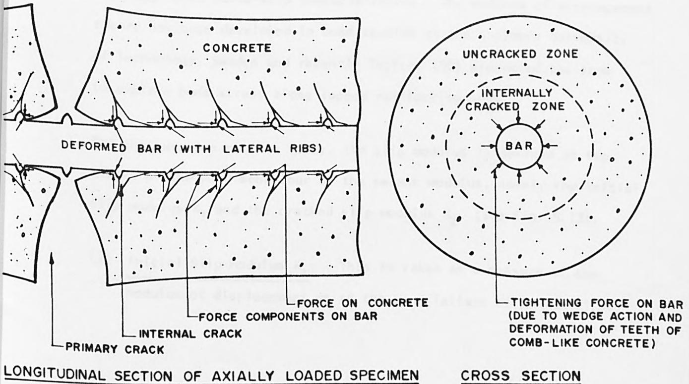
FIG. 5.12 DEFORMATION OF CONCRETE AROUND REINFORCING STEEL AFTER FORMATION OF INTERNAL CRACKS (Schematic Diagram)
