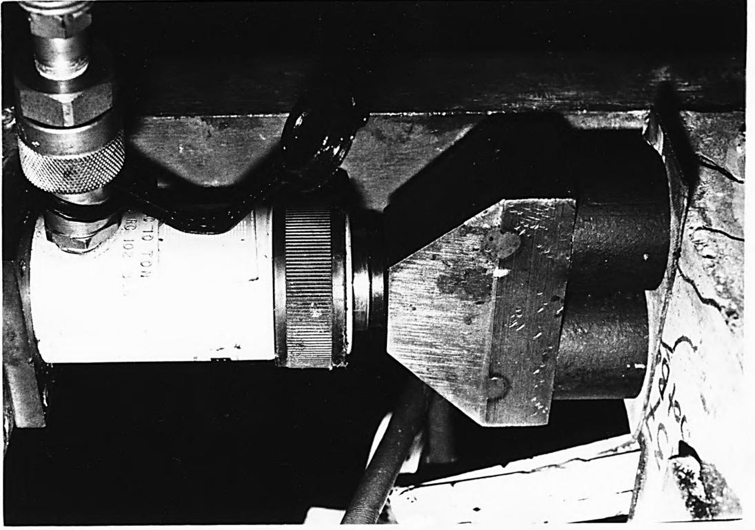
FIG. 4.9 TRANSFER OF LATERAL PRESSURE TO CONCRETE
