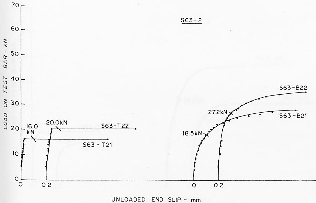
FIG A 27 LOAD-SLIP CHARACTERISTICS AT UNLOADED END - SQUARE-TWISTED BAR
