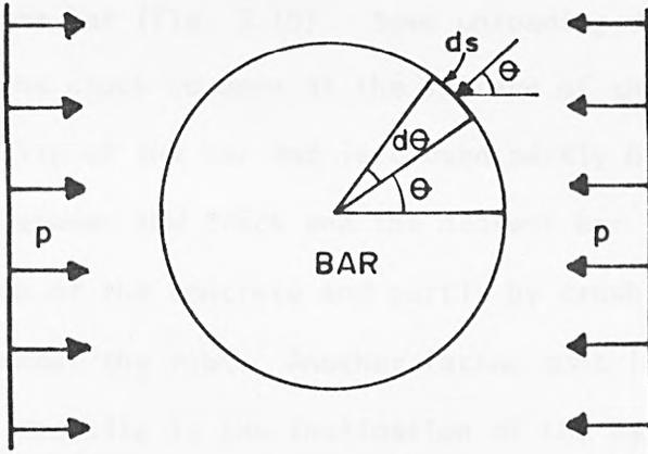
FIG. 5.9 STRESS ON BAR/CONCRETE INTERFACE
