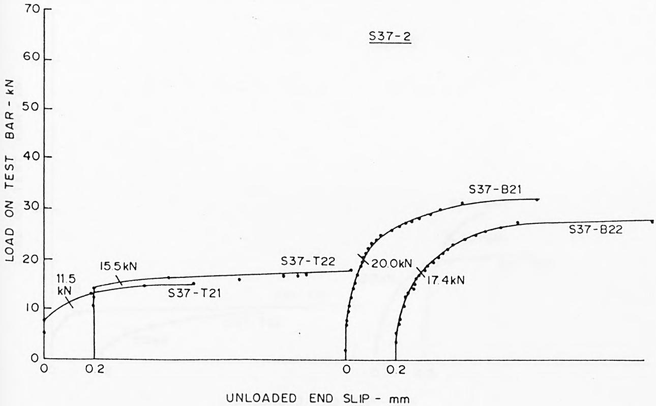
FIG. A 29 LOAD-SLIP CHARACTERISTICS AT UNLOADED END - SQUARE-TWISTED BAR
