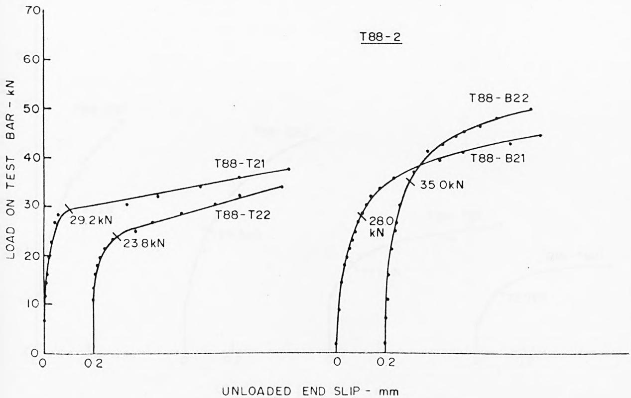
FIG. A.9 LOAD-SLIP CHARACTERISTICS AT UNLOADED END - TORBAR
