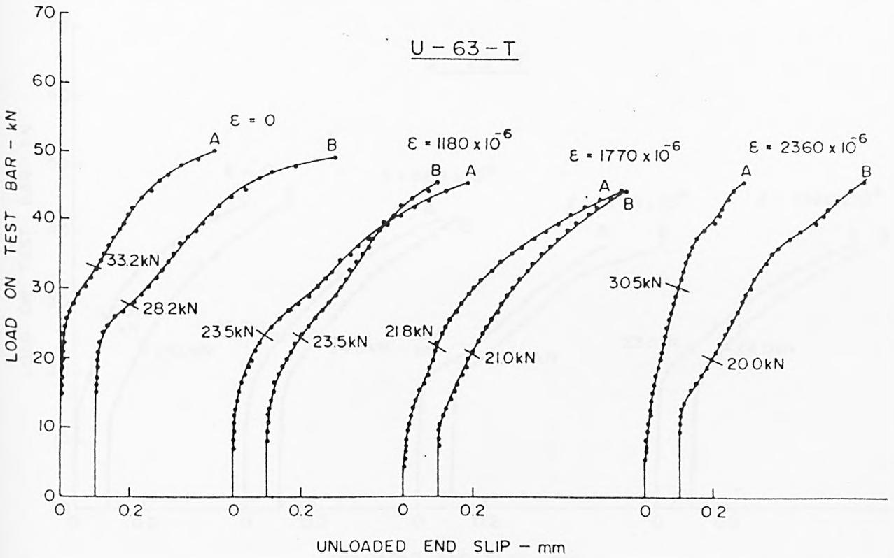
FIG A.3 LOAD-SLIP CHARACTERISTICS AT UNLOADED END - HYBAR
