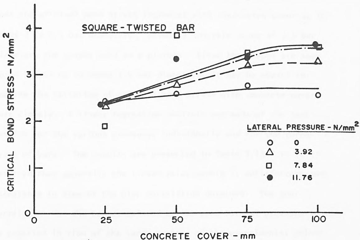
FIG. 7.12 VARIATION OF CRITICAL BOND STRESS WITH CONCRETE COVER - SQUARE-TWISTED BAR
