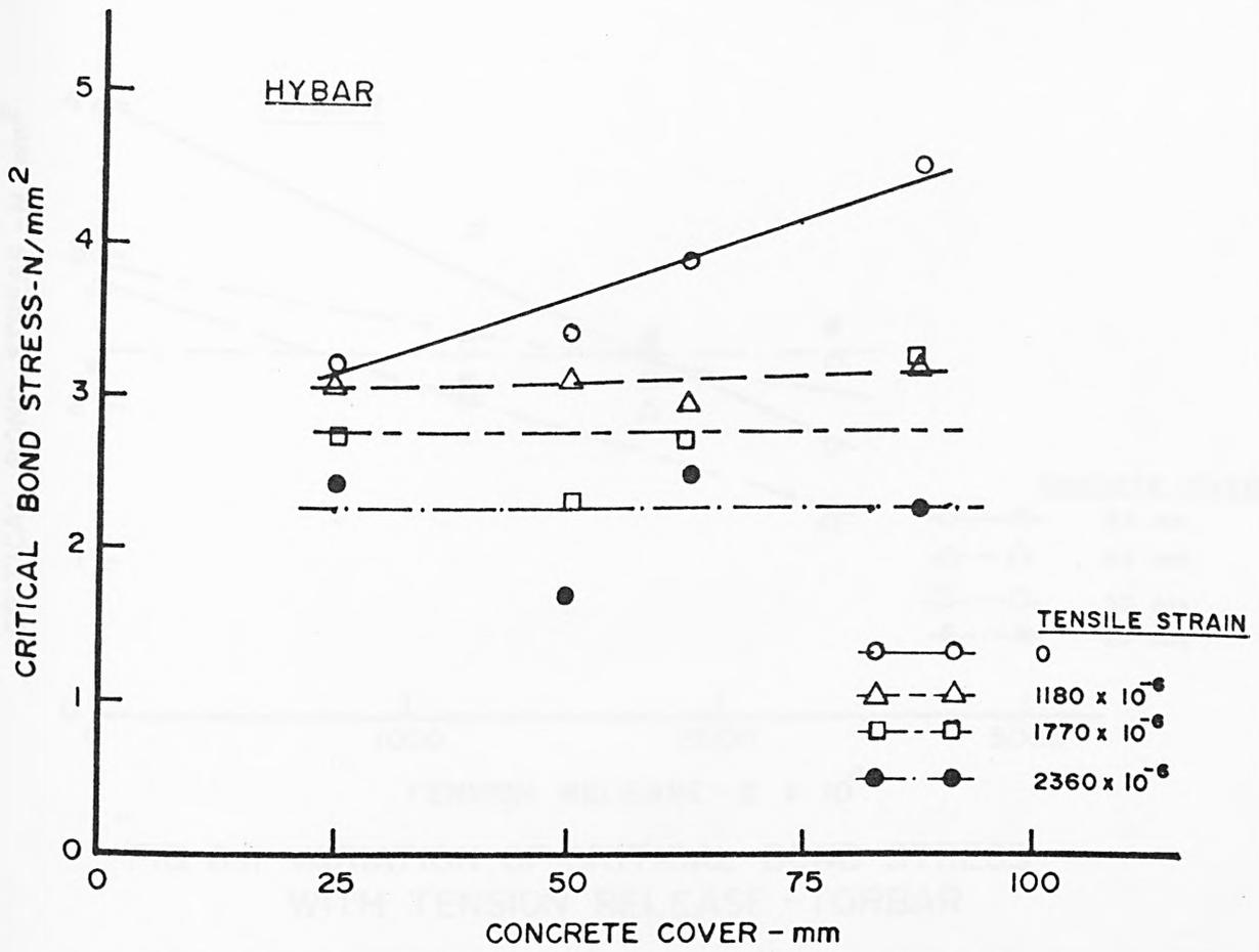
FIG. 6.9 VARIATION OF CRITICAL BOND STRESS WITH COVER - HYBAR
