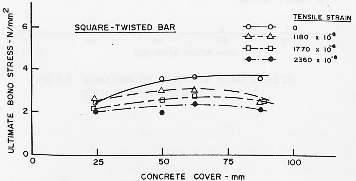
FIG. 6.2 VARIATION OF ULTIMATE BOND STRESS WITH COVER - SQUARE-TWISTED BAR
