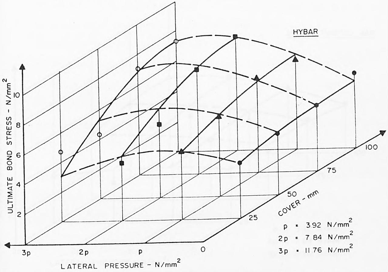
FIG. 78 VARIATION OF BOND STRESS WITH COVER AND LATERAL PRESSURE (Top) CRITICAL BOND STRESS, (Bottom) ULTIMATE BOND STRESS
