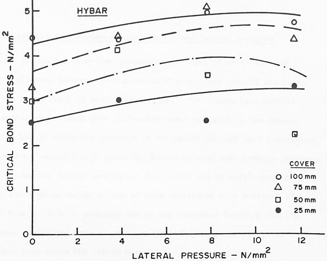
FIG. 7.14 VARIATION OF CRITICAL BOND STRESS WITH LATERAL PRESSURE - HYBAR
