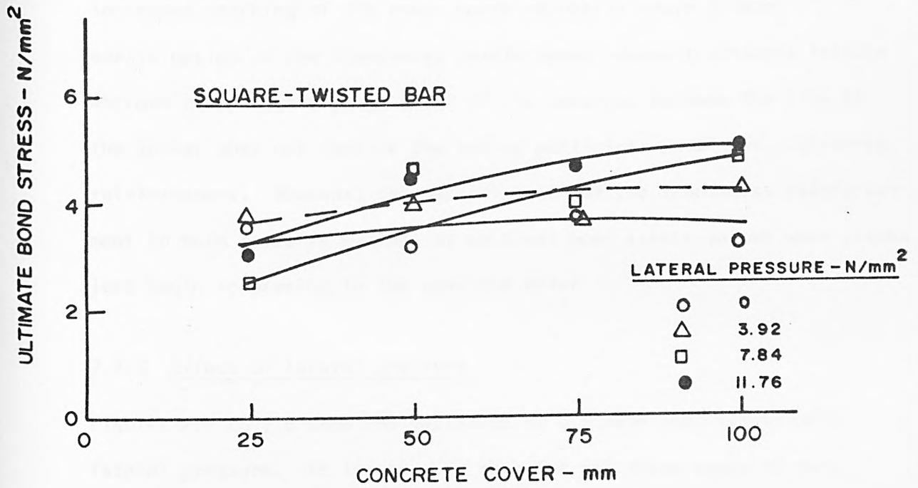
FIG. 7.3 VARIATION OF ULTIMATE BOND STRESS WITH CONCRETE COVER - SQUARE-TWISTED BAR
