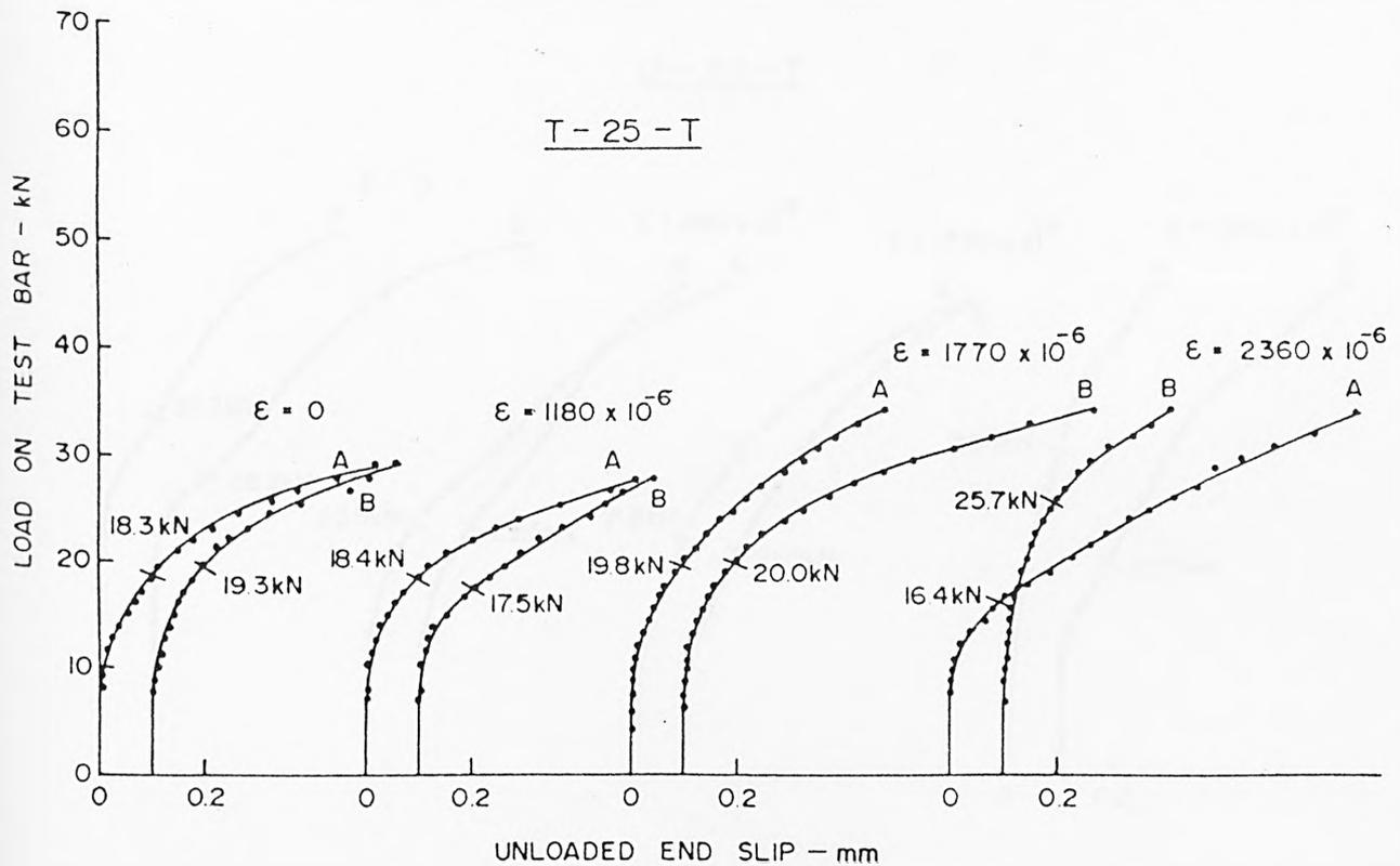
FIG. A2 LOAD-SLIP CHARACTERISTICS AT UNLOADED END - TORBAR
