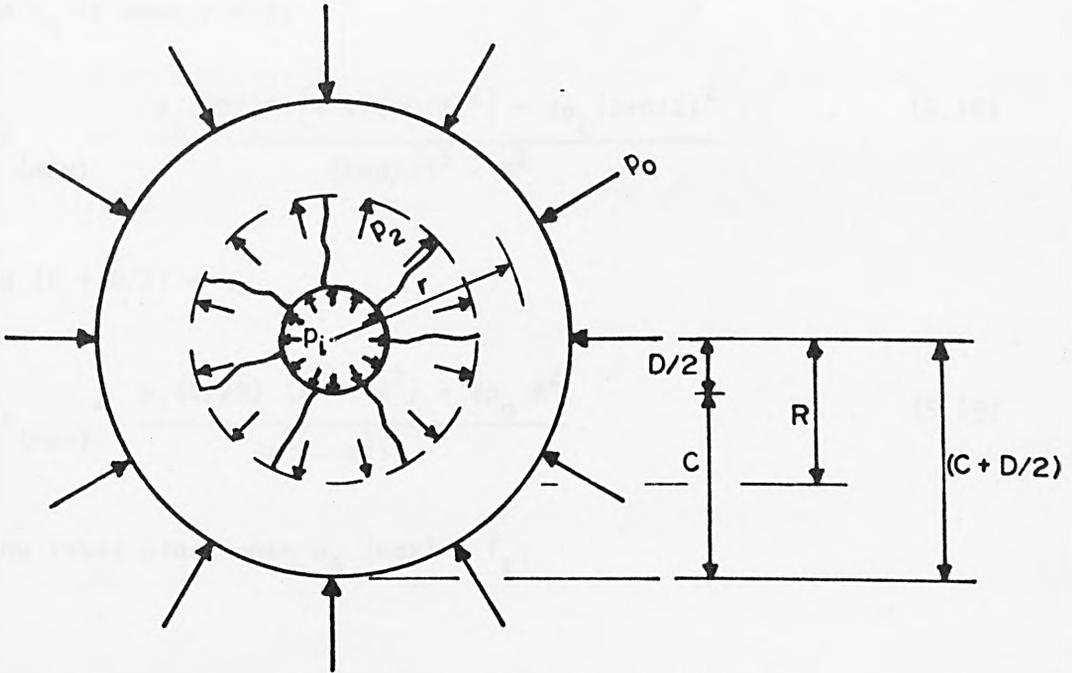
FIG. 5.6 INTERNAL CRACKING IN CONCRETE RING UNDER UNIFORM EXTERNAL PRESSURE
