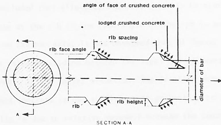
Fig. 2.1: The geometry of a deformed reinforcing bar and the mechanical interaction between the bar and the concrete. (after Rehm)
