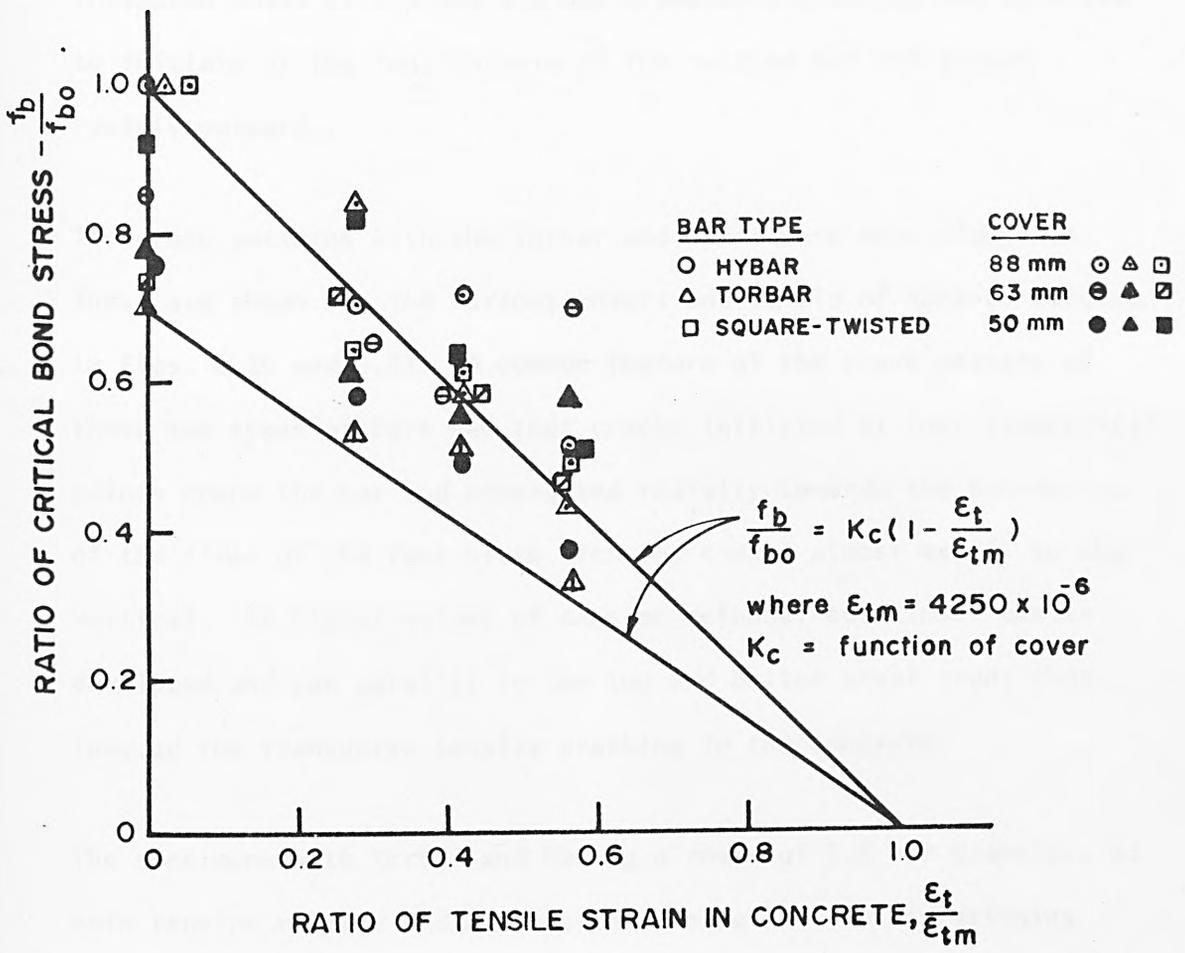
FIG. 6.16 VARIATION OF RATIO OF CRITICAL BOND STRESS WITH RATIO OF TENSILE STRAIN IN CONCRETE
