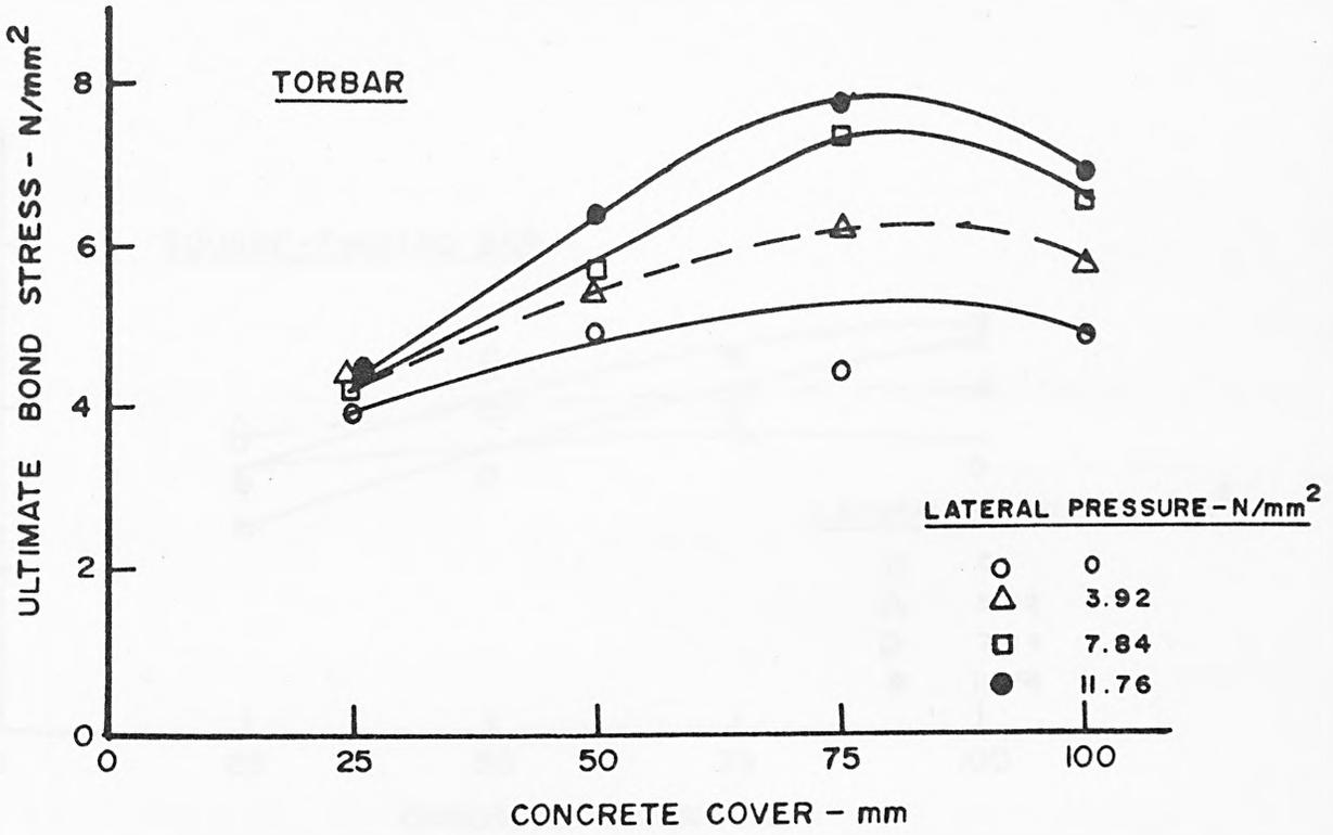
FIG. 7.1 VARIATION OF ULTIMATE BOND STRESS WITH CONCRETE COVER - TORBAR
