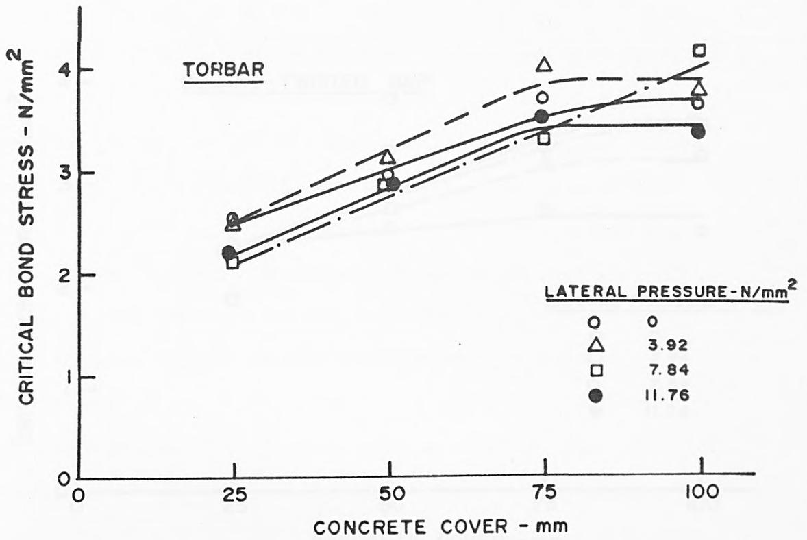
FIG. 7.10 VARIATION OF CRITICAL BOND STRESS WITH CONCRETE COVER - TORBAR
