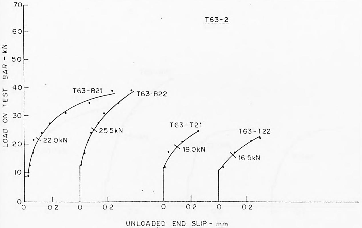
FIG A11 LOAD-SLIP CHARACTERISTICS AT UNLOADED END - TORBAR
