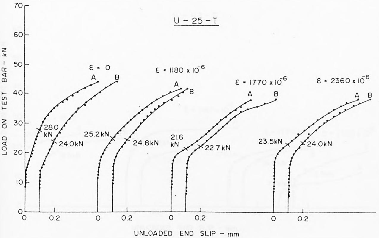
FIG A4 LOAD-SLIP CHARACTERISTICS AT UNLOADED END - HYBAR
