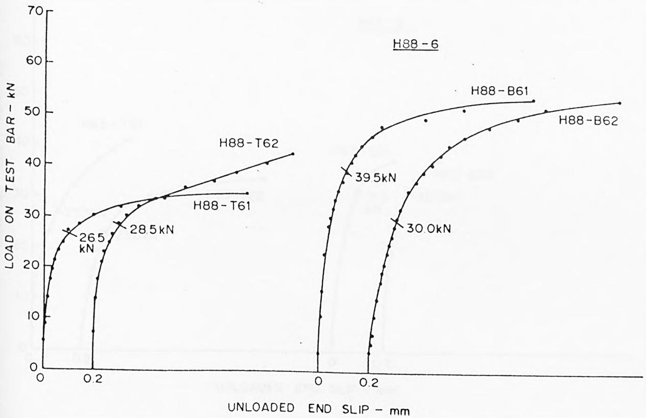
FIG A18 LOAD-SLIP CHARACTERISTICS AT UNLOADED END - HYBAR
