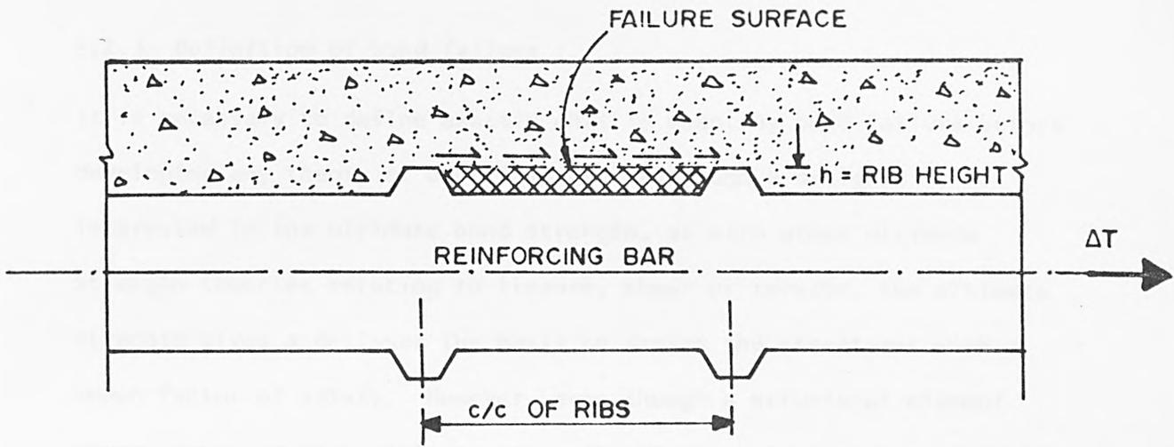
FIG. 5.7 PLOUGH-THROUGH SHEAR MECHANISM
