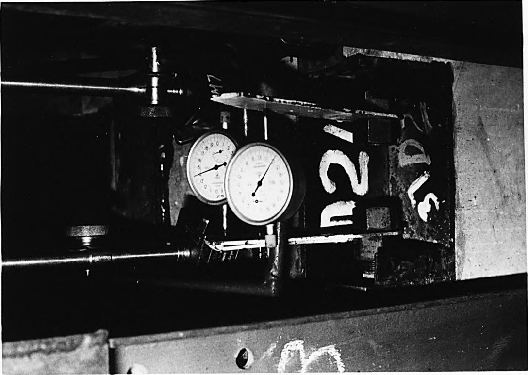
FIG. 4.10 ARRANGEMENT FOR SLIP MEASUREMENT
