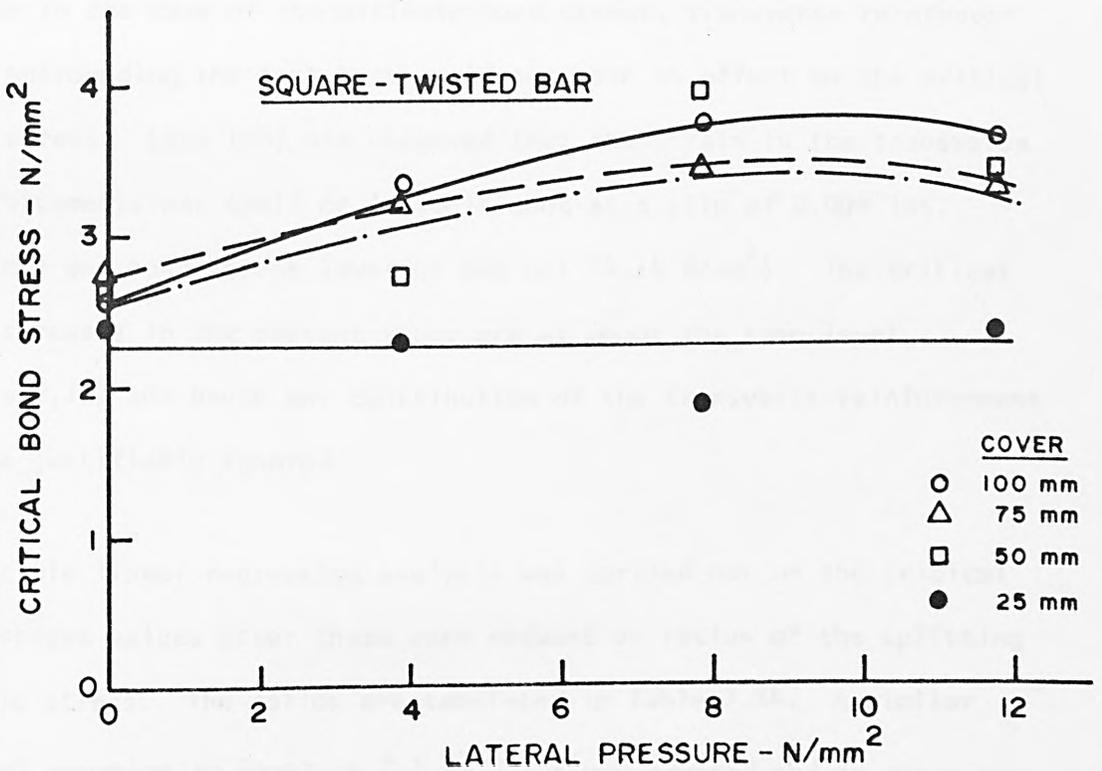
FIG. 7.15 VARIATION OF CRITICAL BOND STRESS WITH LATERAL PRESSURE - SQUARE-TWISTED BAR
