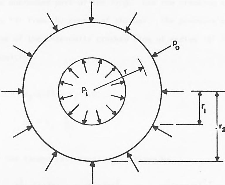
FIG. 5.5 THICK RING UNDER INTERNAL AND EXTERNAL PRESSURE
