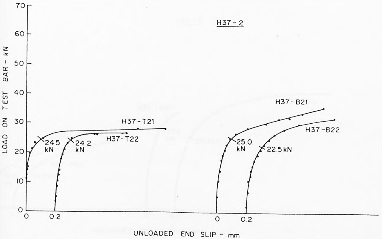
FIG A 21 LOAD-SLIP CHARACTERISTICS AT UNLOADED END-HYBAR
