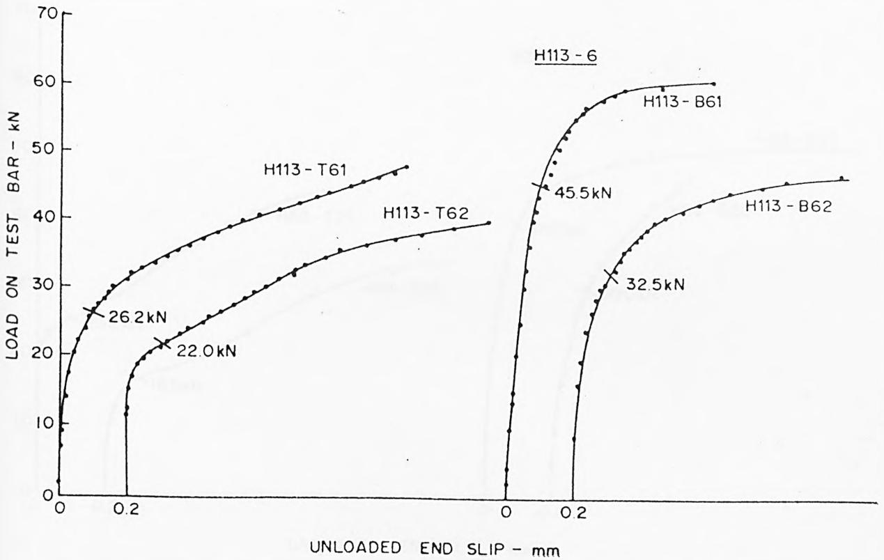
FIG. A.16 LOAD-SLIP CHARACTERISTICS AT UNLOADED END - HYBAR
