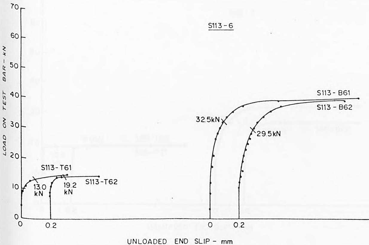
FIG A 24 LOAD-SLIP CHARACTERISTICS AT UNLOADED END - SQUARE-TWISTED BAR
