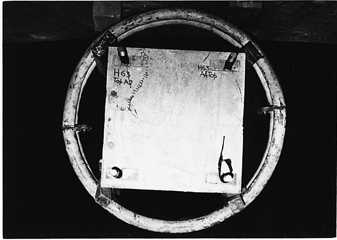
FIG. 4.11 DEVICE FOR ROTATING TEST BLOCK
