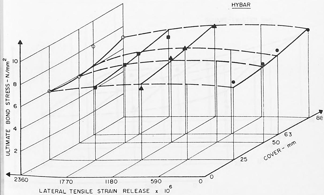
FIG 6.5 VARIATION OF BOND STRESS WITH COVER AND TENSION RELEASE
