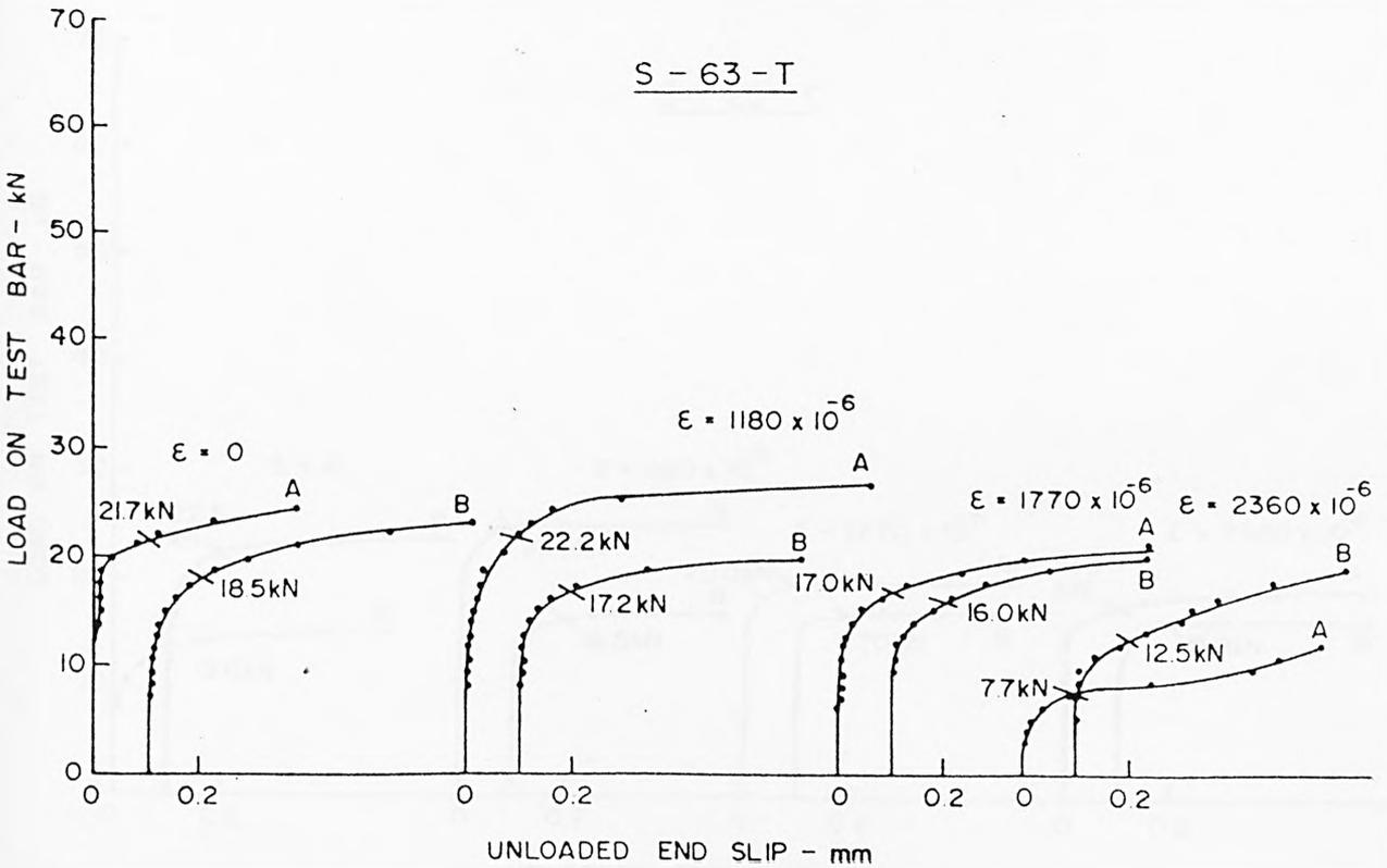
FIG A.5 LOAD-SLIP CHARACTERISTICS AT UNLOADED END - SQUARE-TWISTED BAR
