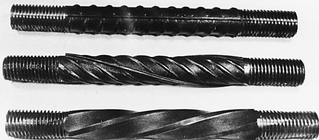
FIG. 3.4 TYPES OF REINFORCEMENT BARS STUDIED
