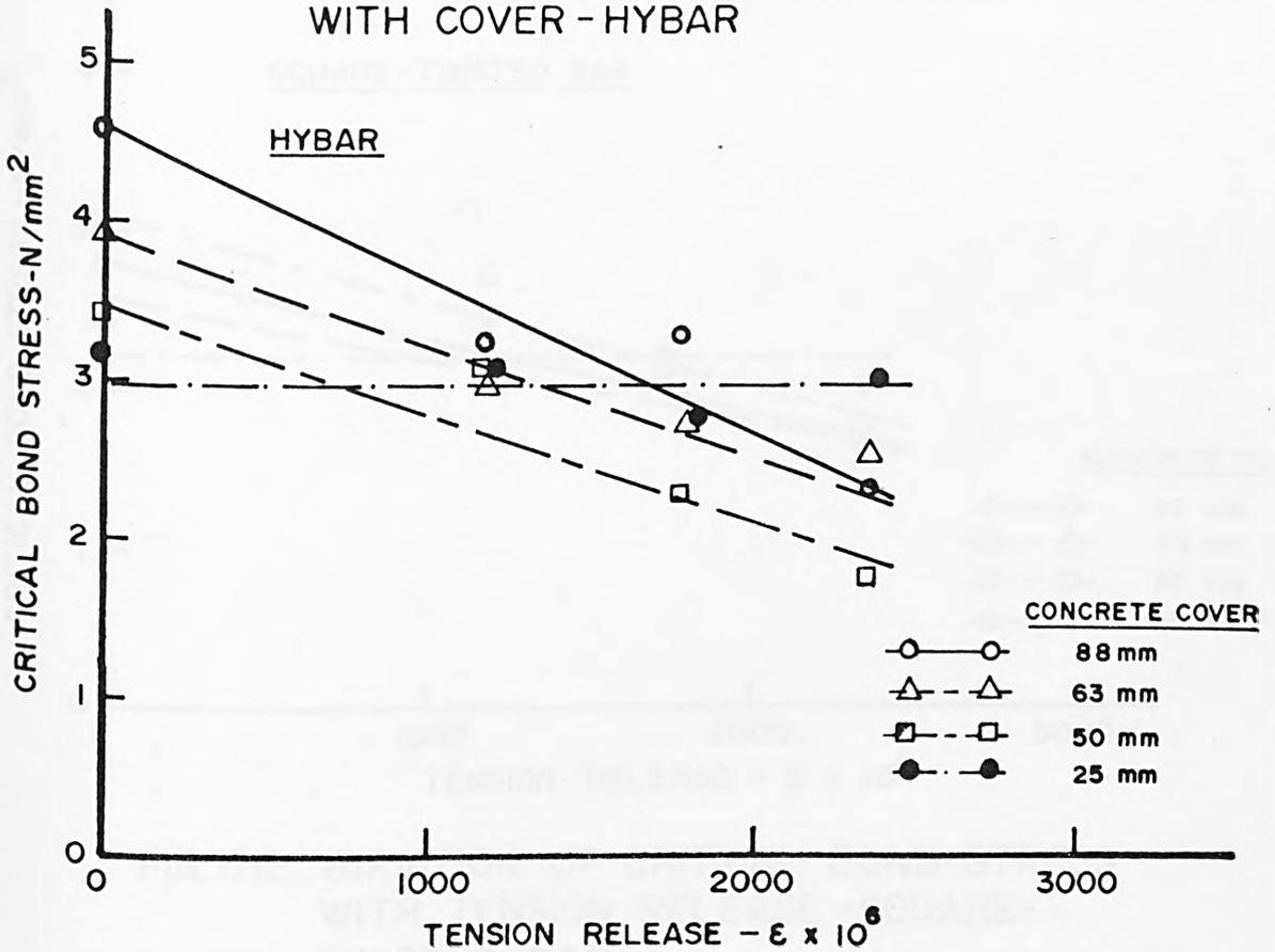
FIG. 6.10 VARIATION OF CRITICAL BOND STRESS WITH TENSION RELEASE - HYBAR
