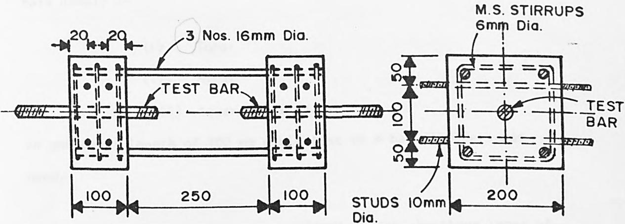
FIG. 3.2 DETAILS OF TEST SPECIMEN - LATERAL TENSION RELEASE
