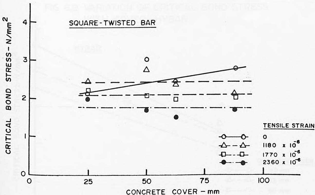
FIG. 6.8 VARIATION OF CRITICAL BOND STRESS WITH COVER - SQUARE-TWISTED BAR
