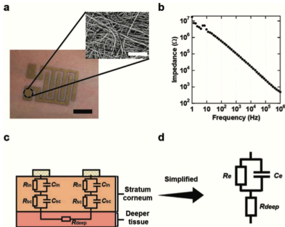
Figure 5.8: Measurement of skin impedance using nanomesh electrodes. a) Optical photograph and SEM image of nanomesh electrode pair attached to the skin, b) measured skin impedance, c) equivalent circuit of human skin, and d) simplified equivalent circuit[74]
