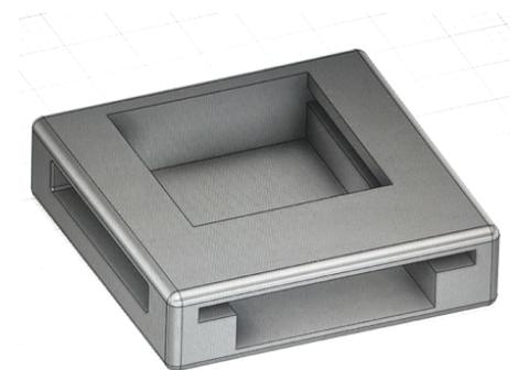
Figure 7.7: 3D-printed casing for PCB and CaF<sub>2</sub> optical window in matte black
