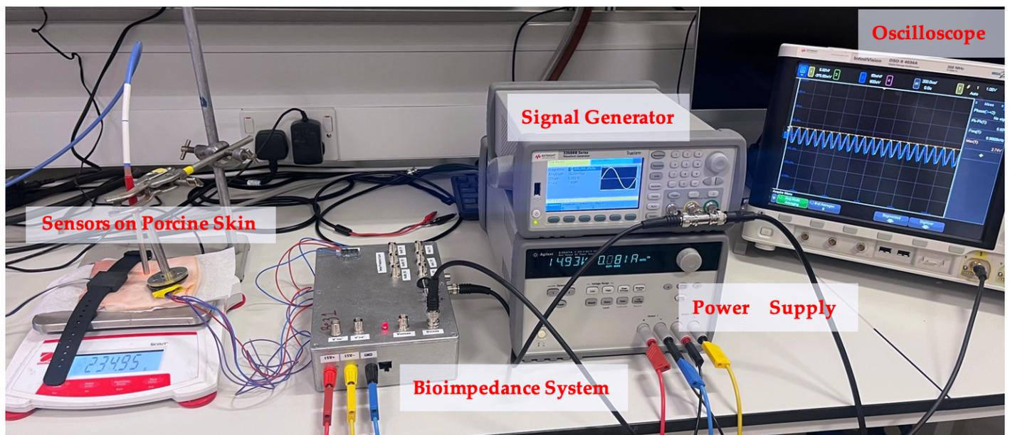
Figure 9.10: Ex vivo experimental setup for bioimpedance system.
