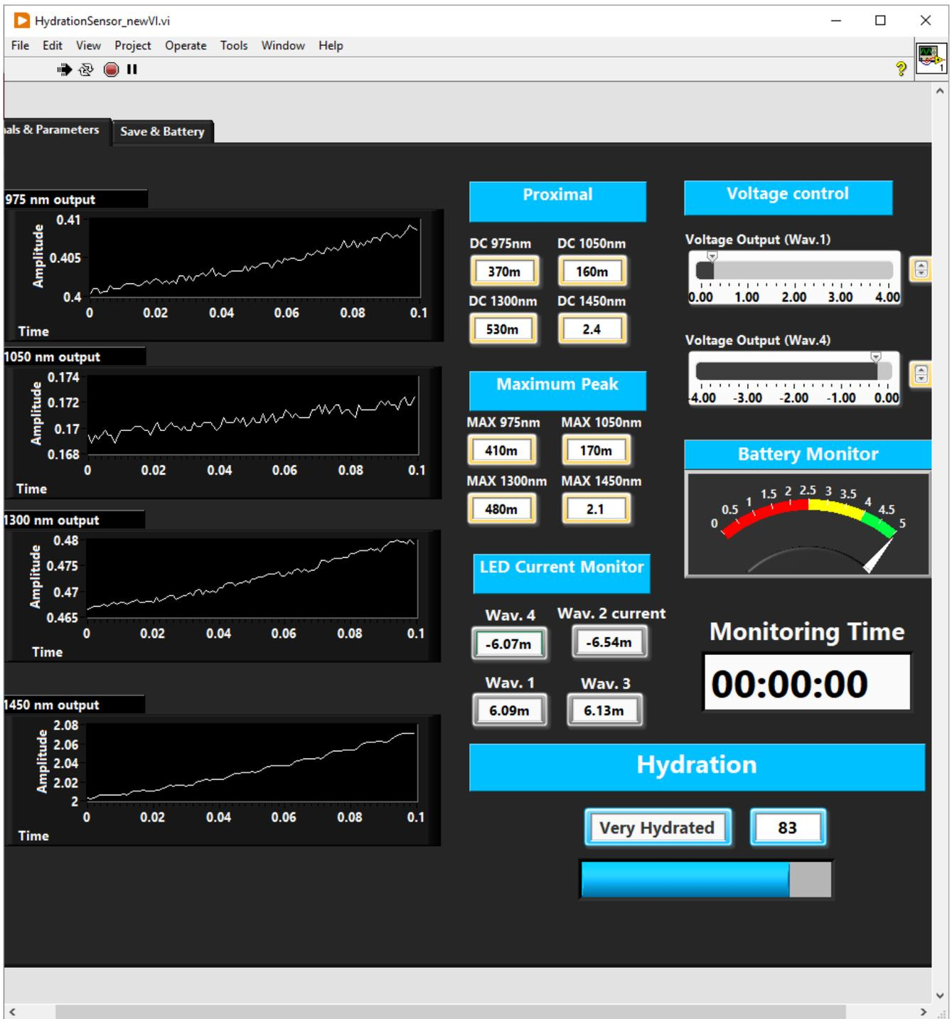
Figure 7.12: LabVIEW front panel for hydration measurements from optical sensor
