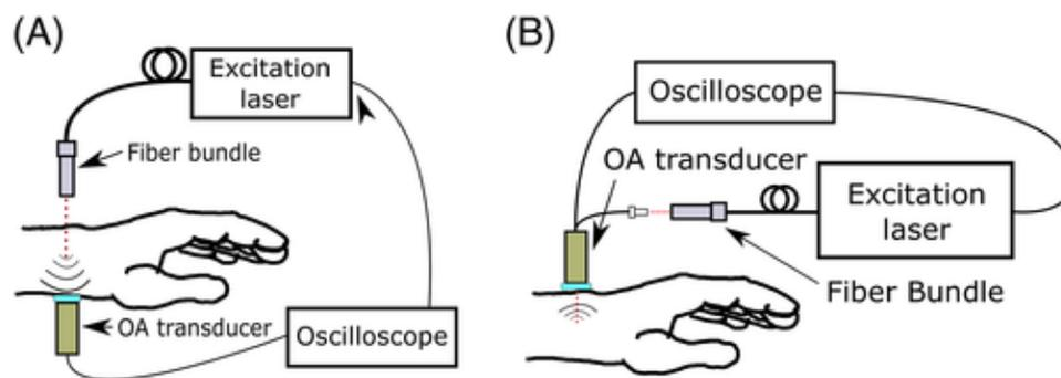
Figure 5.19: Experimental setup for OA measurements in the human wrist in the transmission mode A; and the reflection mode B[85]
