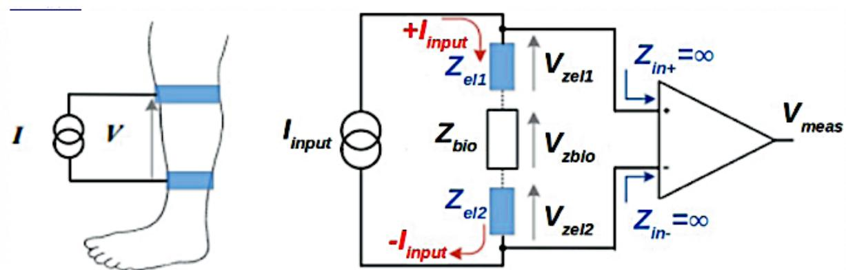
Figure 5.6: Circuit of a bipolar bioimpedance technique, where  $I_{input}$  is injecting current,  $Z_{el}$  is electrode impedance,  $Z_{bio}$  is biological sample,  $Z_{in}$  is input impedance of the measuring amplifier,  $V_{zel}$  and  $V_{zbio}$  are the voltage across the electrode and sample[71]
