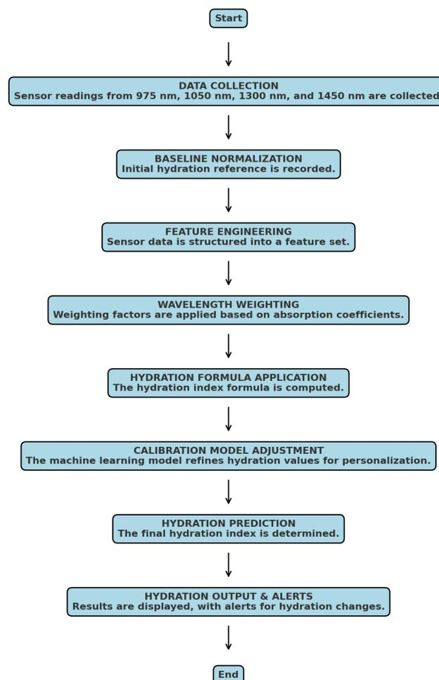
Figure 7.13: Flowchart illustrating hydration monitoring system software process
