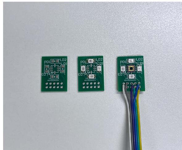
Figure 7.2: PCB with surface-mount LEDs and photodiode soldered
