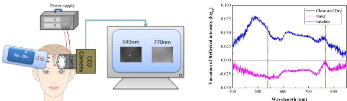
Figure 5.24: left) Experimental setup. right) Variation of reflected intensities between water and Vaseline with respect to clean and dry skin[109]
