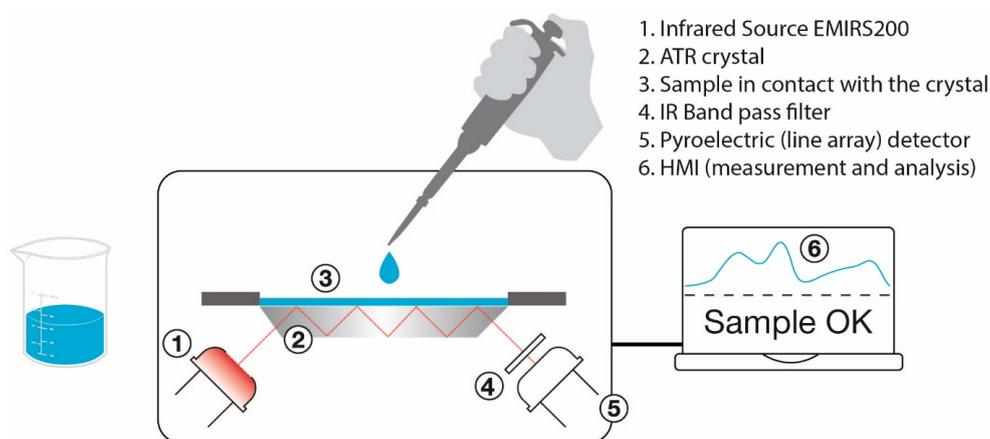
Figure 5.14: Attenuated Total Reflectance Infrared Spectroscopy Measurement Process[80]
