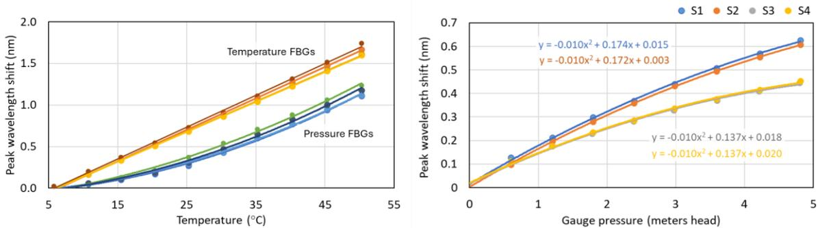
Figure 2. (left) Response of both FBGs of Sensor 1 vs temperature. (right) Response of the pressure sensitive FBGs of all four sensors versus pressure (50µm diaphragm (S1, S2) and 100µm diaphragm (S3, S4)).
