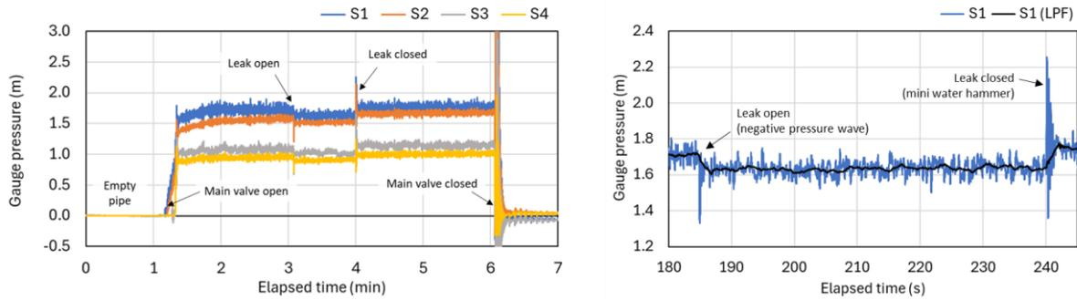
Figure 3. (left) Pipe pressure at the different sensing locations for an exemplary test cycle. (right) Pressure drop and transient signatures caused by a leak of 12mm in diameter. Blue line (raw data); Black line (low-pass filtered, 2<sup>nd</sup> order Butterworth, 0.1Hz).
