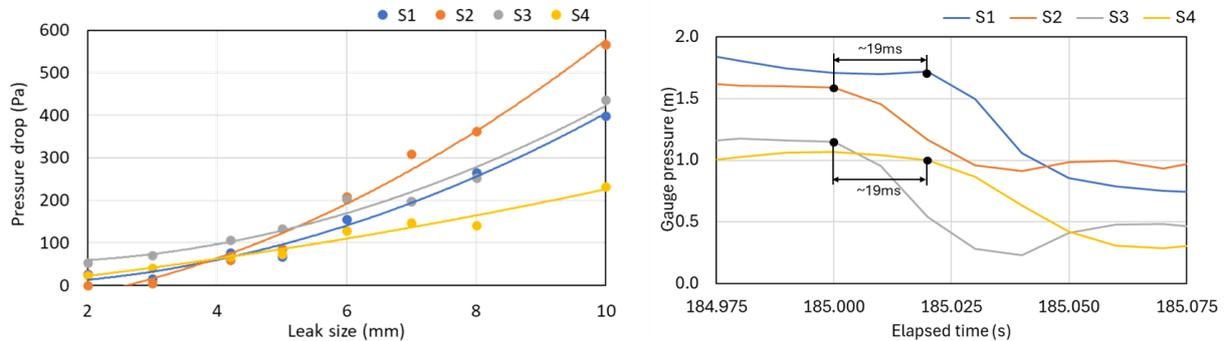
Figure 5. (left) Pressure drop vs leak size. Leaks down to 2mm in diameter were successfully identified. (right) Time delay in the response of the sensors further away from the leak (S1 and S4) to those closer to the leak (S2 and S3).
