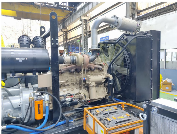
(c) Compressor block connected to diesel engine
