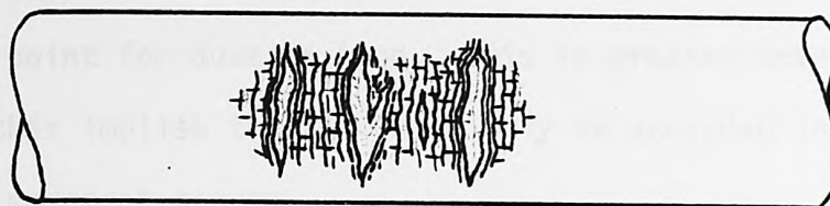
FIG. 2.9 Graphitic fissures on surface of pipe
