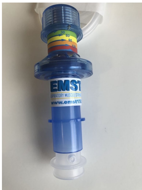
FIGURE 4 | Device with modified In-Health manometer adapter.
