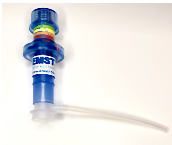
FIGURE 5 | Device with In-Health manometer adapter tubing.
