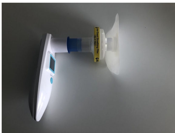
FIGURE 1 | Attachment of PF/FEV1 meter to baseplate.
