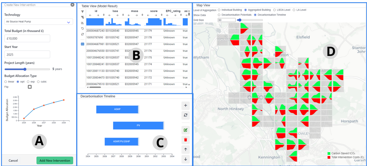
Figure 1: The Decarbonisation Planner Dashboard. In New Intervention Panel (A), users define a granular decarbonisation intervention technology, targeted to specific buildings selected based on socio-demographic considerations, decarbonisation potential, and the geospatial parameters in Table (B) and Map (D) View. The Timeline View (C) allows users to refine modular interventions and adjust scenarios. Finally, (D) shows both multivariate decarbonisation potential and output timelines as glyph maps at different aggregation levels ( https://decarb-vis.netlify.app ).
