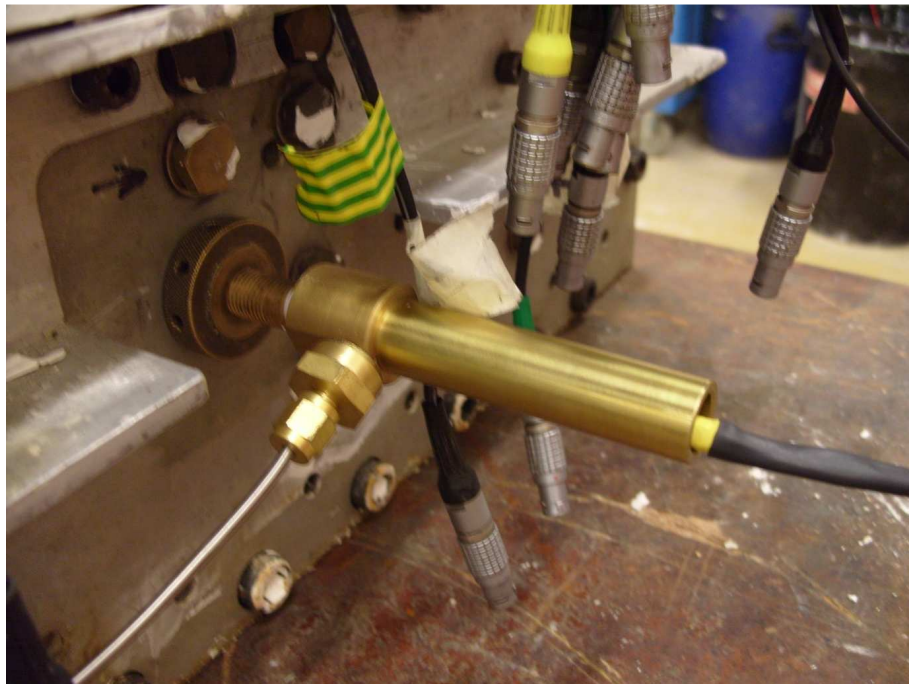
Figure 7.4: Holding nut for securing the tunnelling supporting system in place and the manifold for the tunnel pressure transducer
