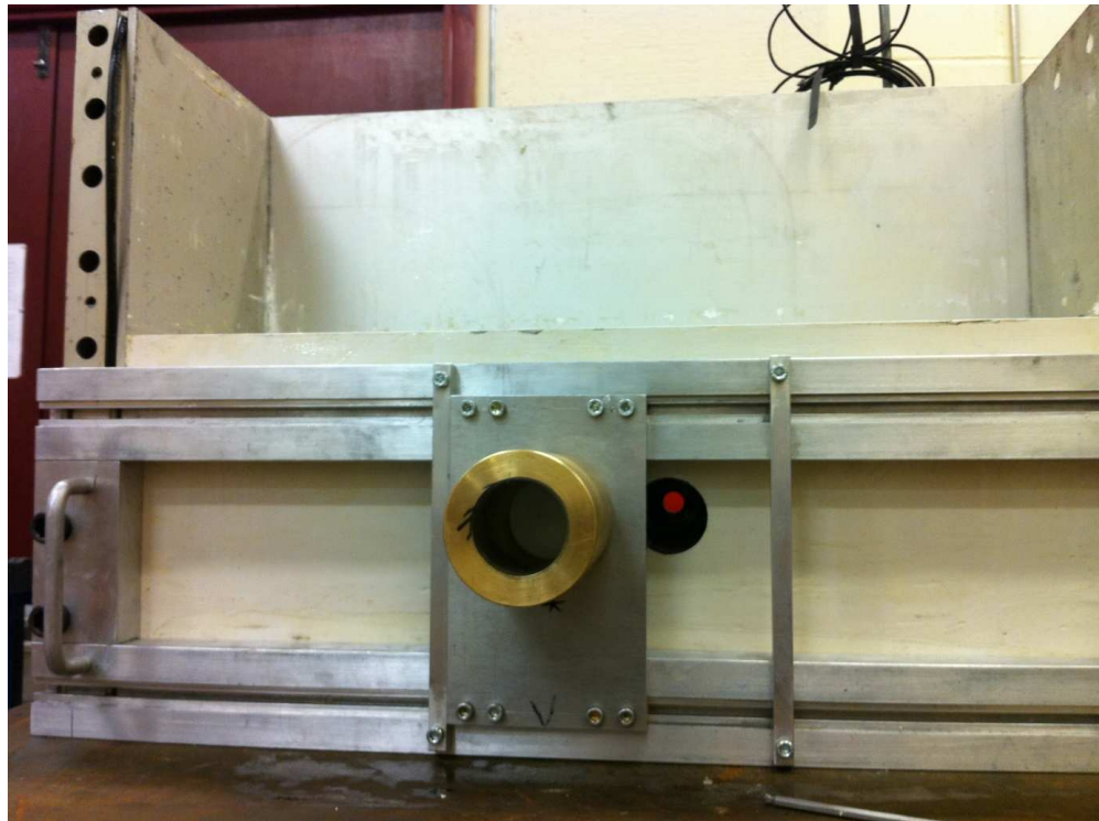
Figure 7.2: Jig for the creation of the twin-tunnel cavities on the bench during the model making stages of centrifuge modelling
