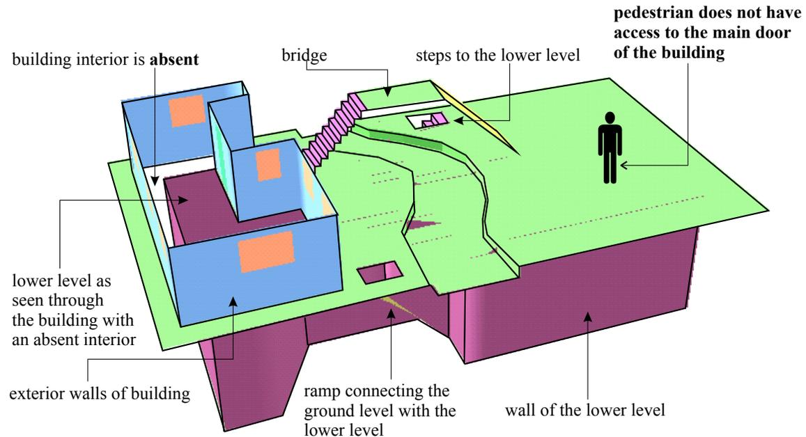
**Figure 4:** The space accessible by a pedestrian without a key from outside the building, out of office hours (according to the access rules shown in Figure 1). Since access to the main door is not allowed, the interior of the building is absent as is the upper storey, because no access can be gained to the internal staircase.
