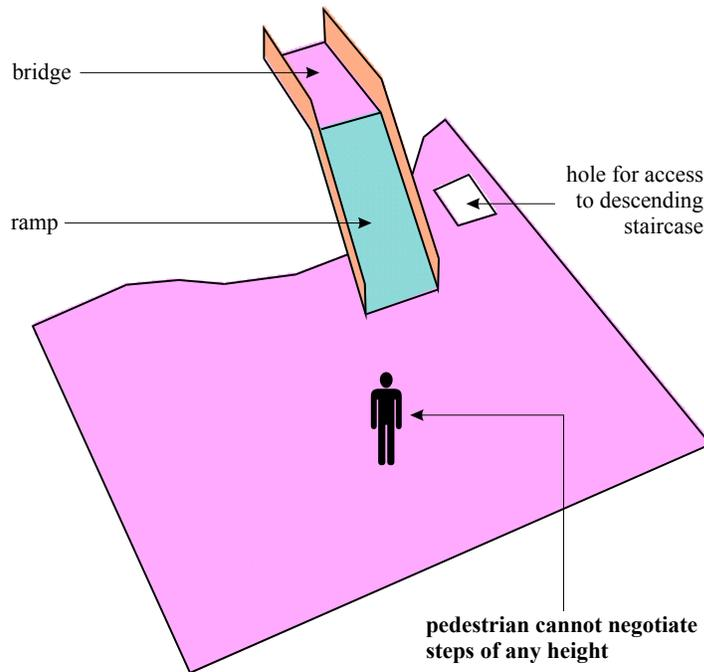
**Figure 6:** This Figure shows the space accessible to a pedestrian who starts on the opposite side of the road to that in Figure 5 and cannot negotiate steps of any size. Note that most of the bridge is accessible from this side of the road because this side is a ramp, but there is no access over the bridge. Also note that there is no lower level because access to this from this side of the road is by a staircase.
