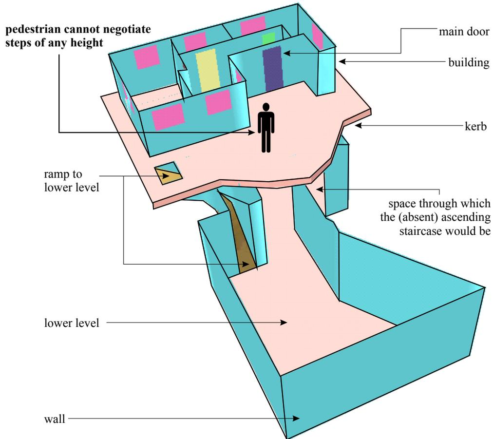
**Figure 5:** This shows the space accessible to a pedestrian who starts just outside the building and cannot negotiate steps of any size. Note that all steps are absent; the road, the other side of the road, the bridge and the upper storey of the building are missing because they can only be accessed either by stairs or steps. All elements shown can be accessed without any steps.
