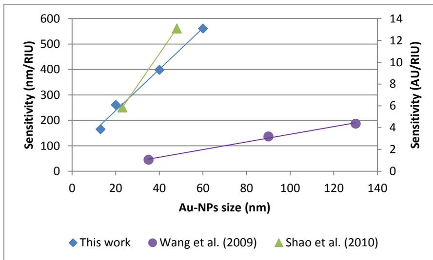
Figure 4.8: Sensitivity comparison of the results from this work with those reported from several examples in the literature. This work and the one of Shao *et al.*'s sensitivities were presented in nm/RIU, while the work from Wang *et al.* was recorded in AU/RIU.
