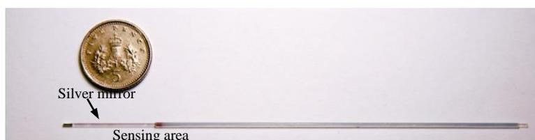
Figure 7.1: Photograph of a sensing probe created, with its size comparing with a 5 pence coin.
