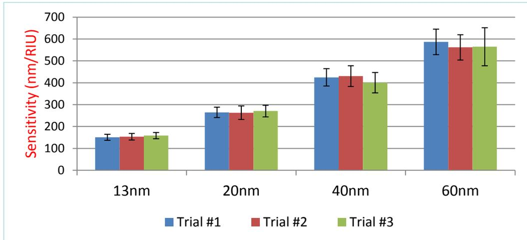
Figure 4.7: Sensitivity comparison of 4 groups of sensors coated with different sizes of AuNPs
