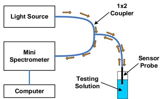
Figure 5.6: Schematic diagram of a typical LSPR sensor system.
