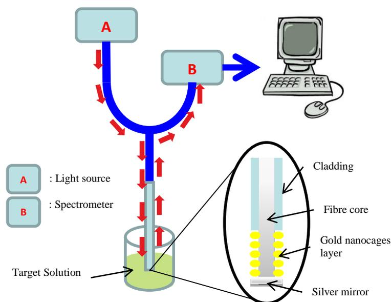
Figure 7.2: Schematic illustration of a LSPR sensor system
