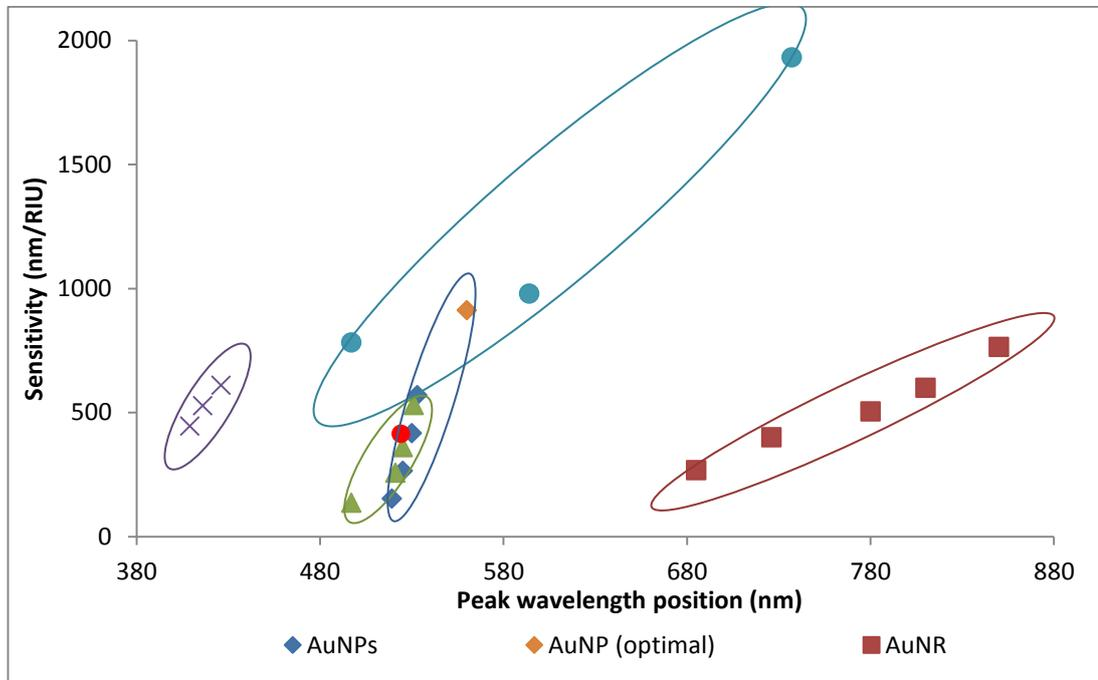
Figure 7.9: Plot of sensitivity vs. plasmonic peak of different gold nanostructures. AuNPs: Gold nanospherical particles; AuNRs: Gold nanorods; AuNCs: Gold nanocages particles; A25, A75 Alloy: Gold/silver alloy nanospherical particles with 25% and 75% Ag content, respectively.
