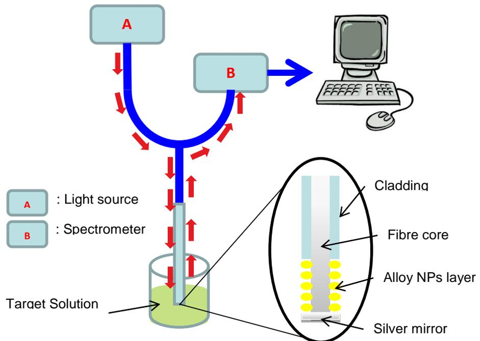
Figure 6.2: Schematic diagram of an experimental setup used in this work
