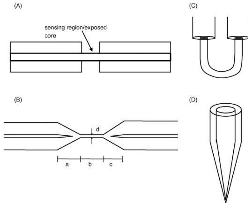
Figure 3.13: Common fibre configurations used in sensing. Reproduced from Ref. [179] © Elsevier 2007
