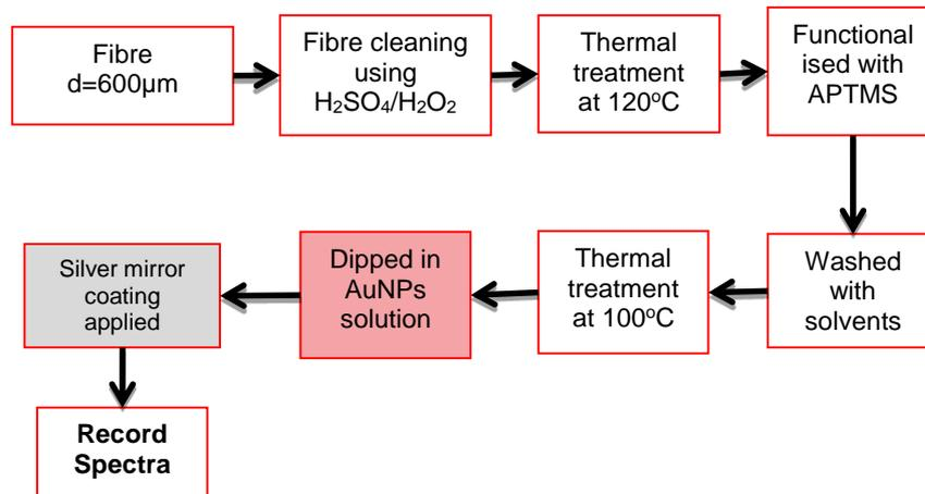
Figure 4.1: Schematic procedure for the coating process
