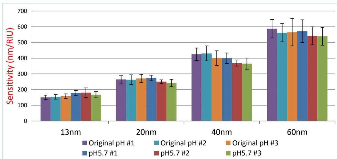
**Figure 4.10: Sensitivity comparison before and after the pH adjustment.**
