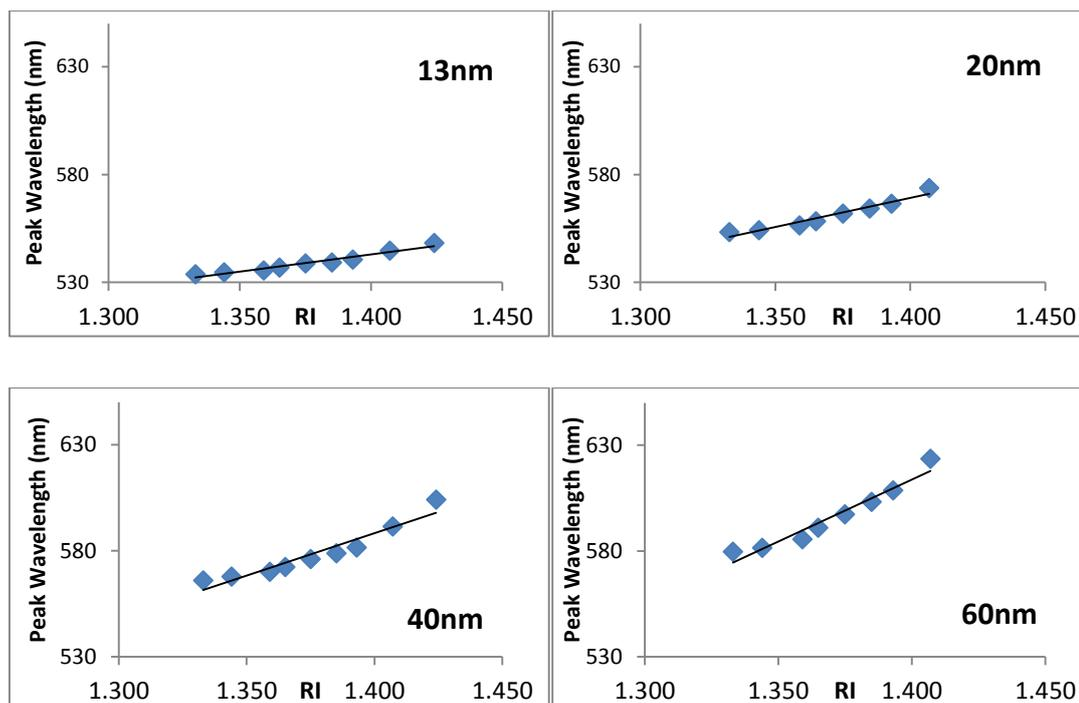
Figure 4.6: Plot of peak wavelength vs. RI value for 4 sensor probes coated with different sizes of AuNPs, i.e. 13nm, 20nm, 40nm and 60nm respectively.
