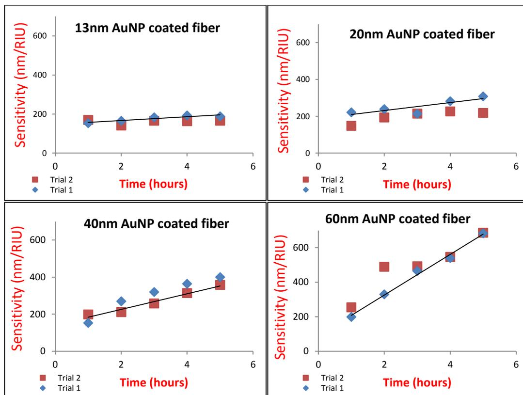
Figure 4.11: Effect of coating time on sensitivity for 4 different AuNP coated fibres with two trials each
