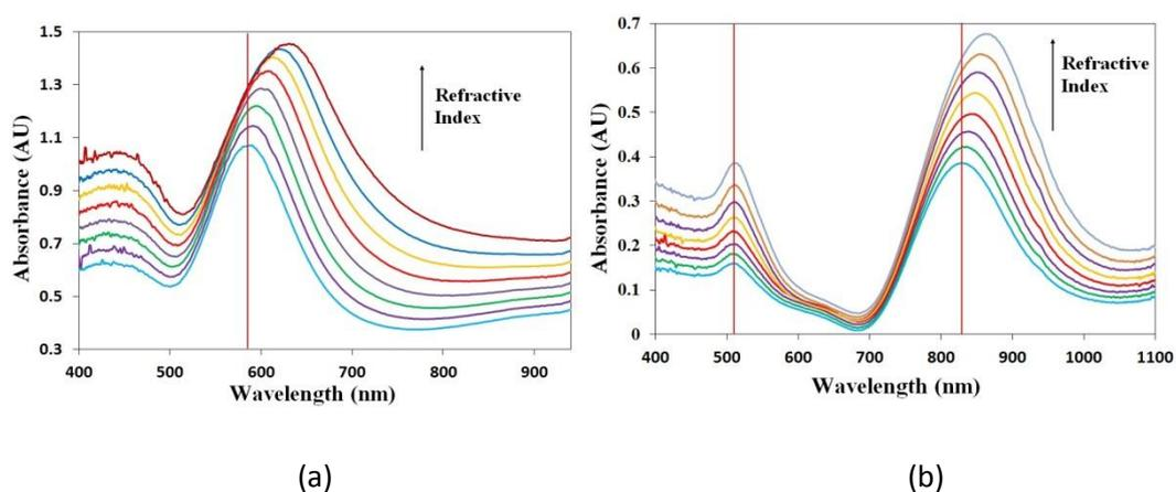
Figure 5.8: Absorbance spectra of (a) 60 nm AuNP-based LSPR sensor, (b) AuNR-based LSPR sensor with an aspect ratio of 4.1, both showing an increase with the increase of the refractive index of the testing solutions.
