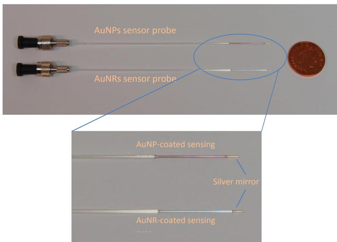
Figure 5.4: Photographs showing the AuNP- and AuNR- coated sensor probes developed in this work.
