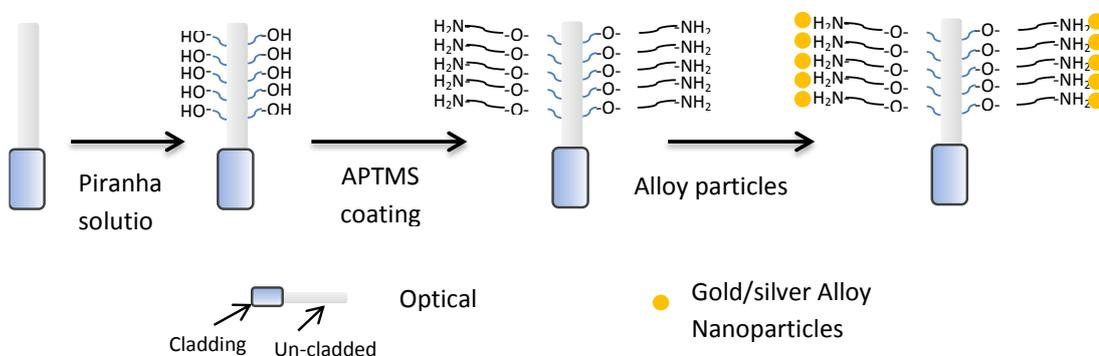
Figure 6.1: Illustration of the preparation of the fibre optic sensor
