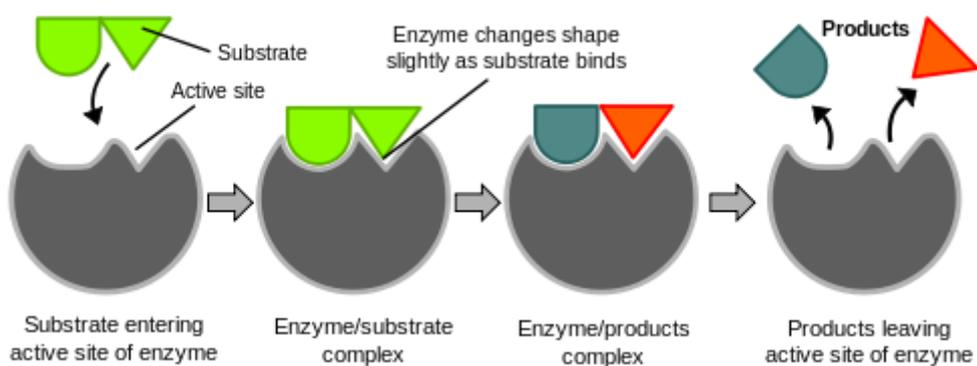
Figure 3.6: "Lock and Key" mechanism of Enzyme catalyst. Reproduced from Ref. [119]
