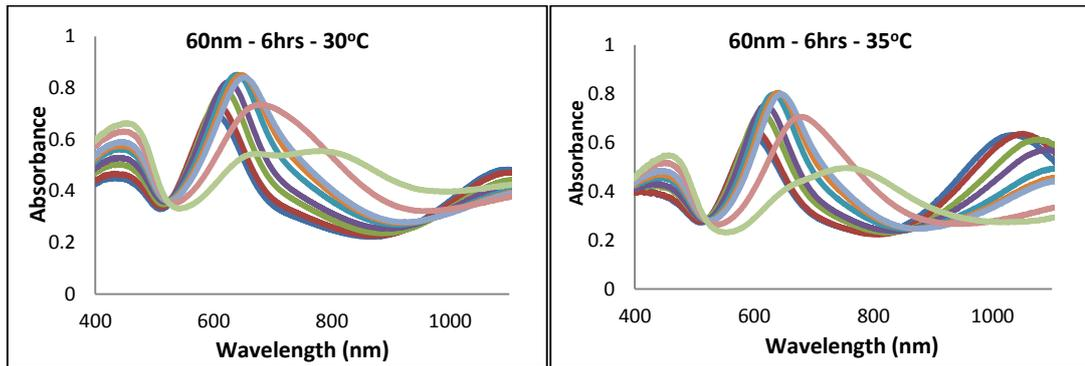
c) 6 hours coating, 60nm AuNP, 30°C coating temp.
