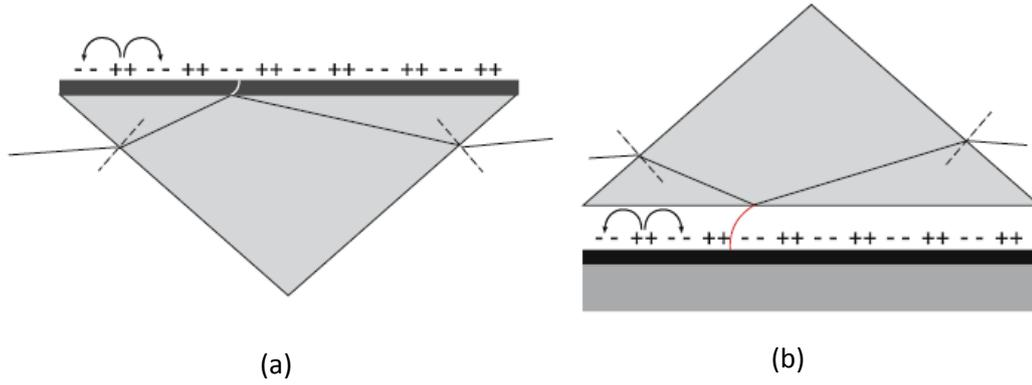
Figure 2.2: (a) Krestchmann and (b) Otto configurations for SPR effect. Reproduced from Ref. [10] © Springer 2007.
