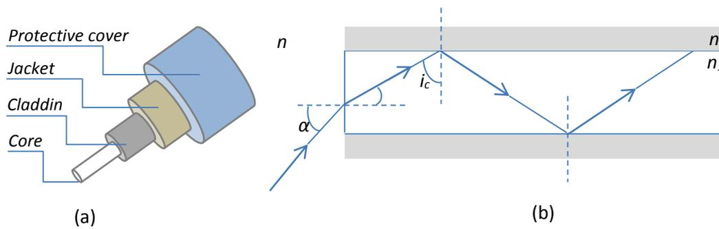
**Figure 2.1: a) Typical fibre structure and b) Total internal reflection inside a fibre core.**
