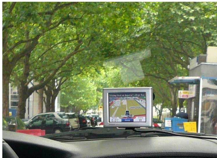
Figure 1.2-2: Free-standing after-market in-vehicle navigation unit (from Garmin™)
