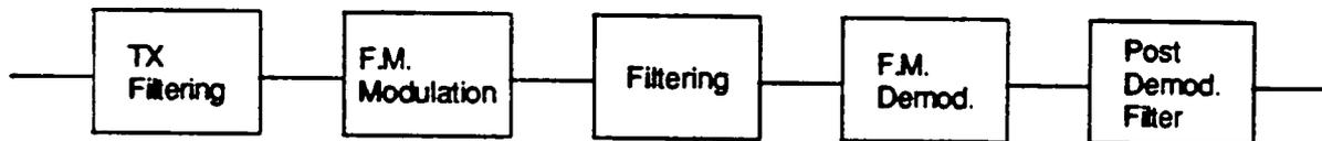
Figure 2.3: Simplified system model used as basis of simulation
