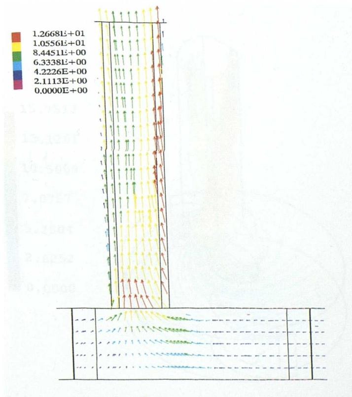
Figure 5.79 Scroll-Compressor. Rotational speed 1000 RPM, Speed vectors, Arbitrary plane, step=100, 50 degrees (8.333m sec) after discharge commences
