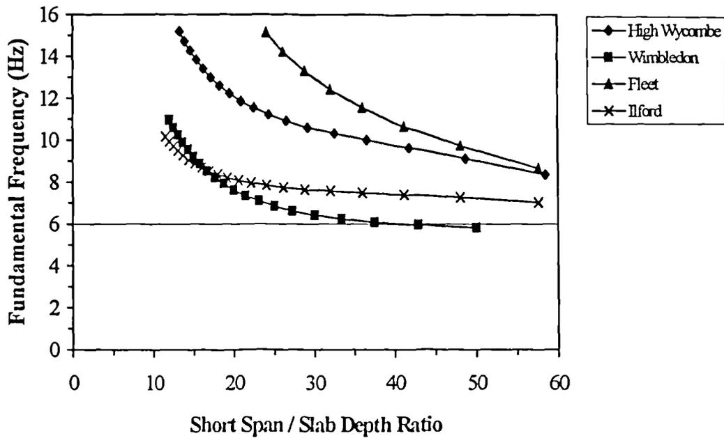
Figure 4.9: Frequency vs Short Span/Depth Ratio
