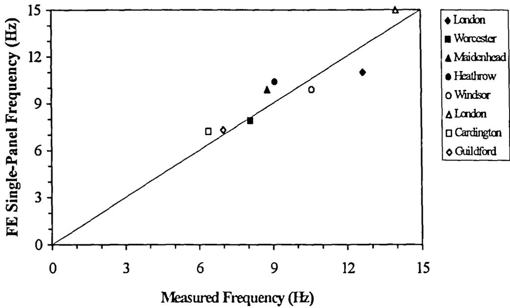
Figure 4.24: Field vs FE Frequency
