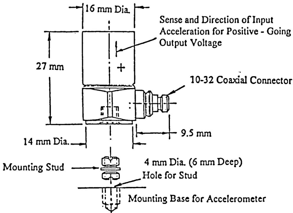
Figure 2.9: Accelerometer Details
