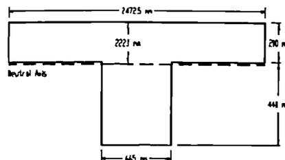
$$\text{Fundamental natural frequency} = \frac{\pi}{2} \sqrt{\frac{EI}{\rho AL^4}} = 7.43 \text{ Hz (simple supports)}$$
