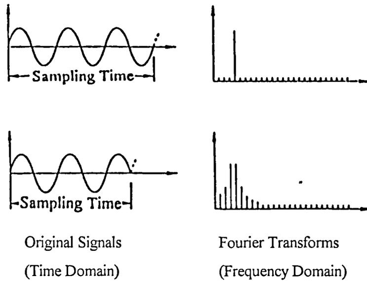
Figure 2.4: Leakage
