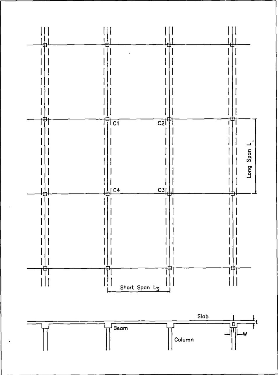
Figure 3.1: Typical Plan Layout and Cross-Section
