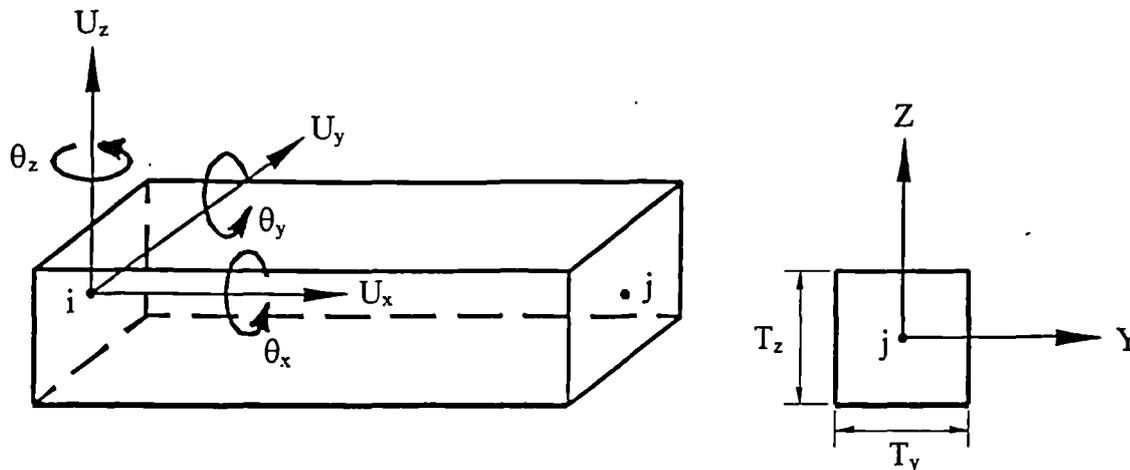
Figure 4.2: Beam Element
