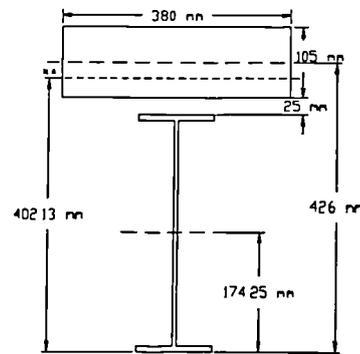
$$\text{Effective slab width} = \text{least of } 0.4 L_b \text{ or } S_b = 2.665 \text{ m}$$
