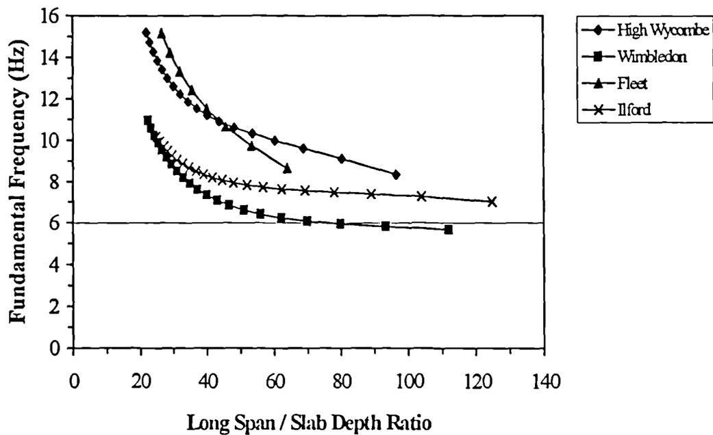
Figure 4.10: Frequency vs Long Span/Depth Ratio
