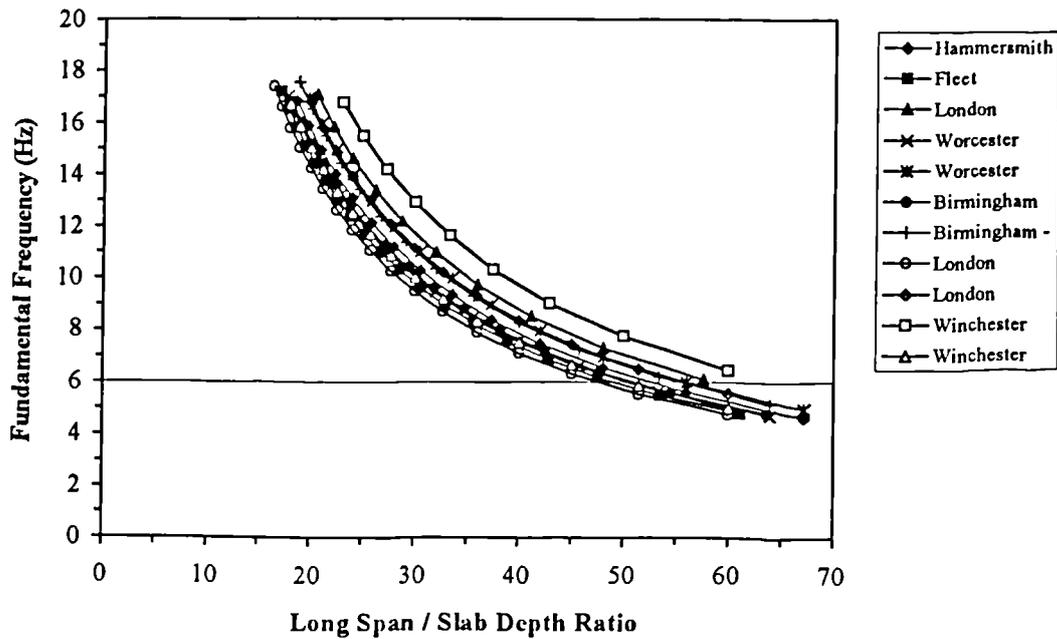
Figure 4.17: Frequency vs Long Span/Depth Ratio
