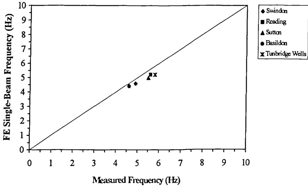
Figure 4.19: Field vs FE Frequency
