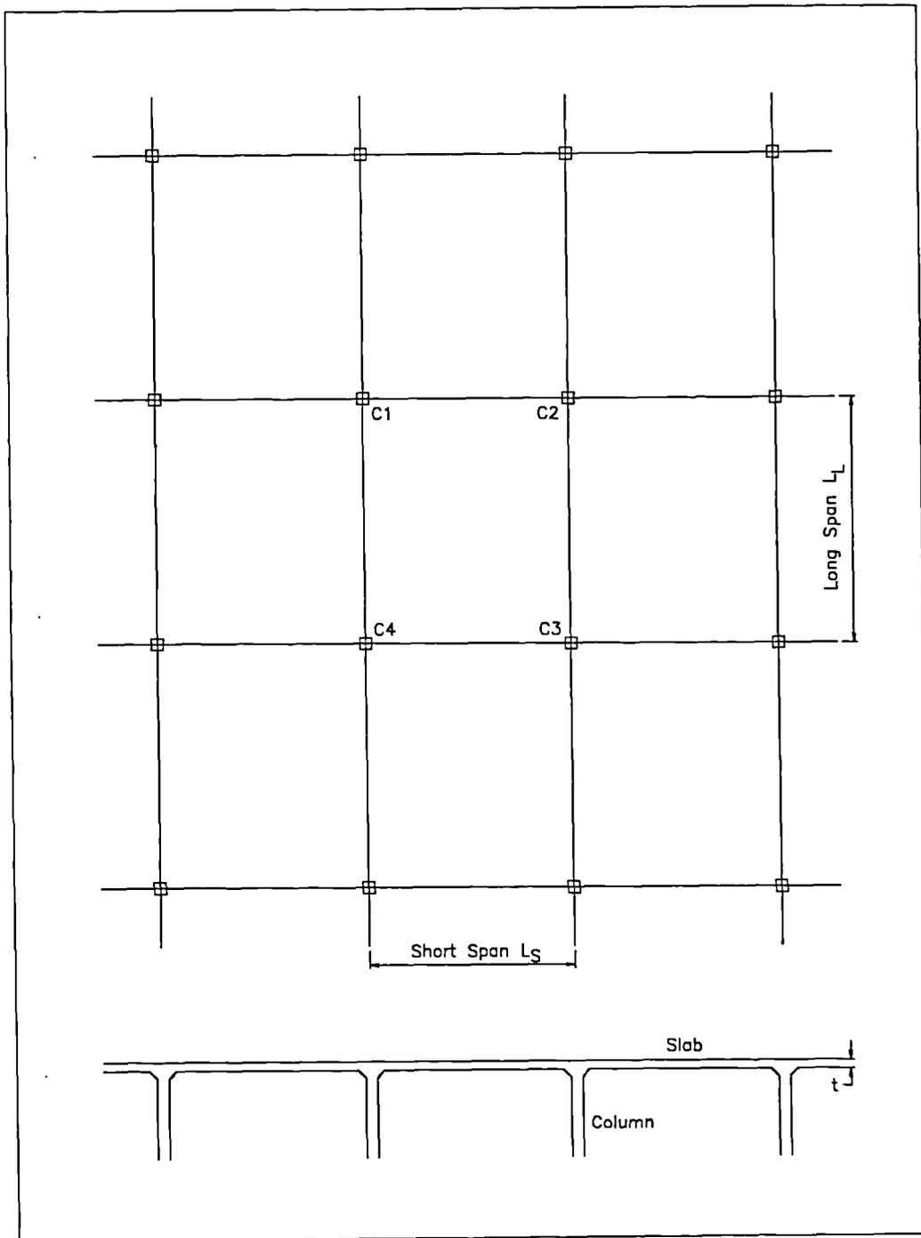
Figure 3.6: Typical Plan Layout and Cross-Section
