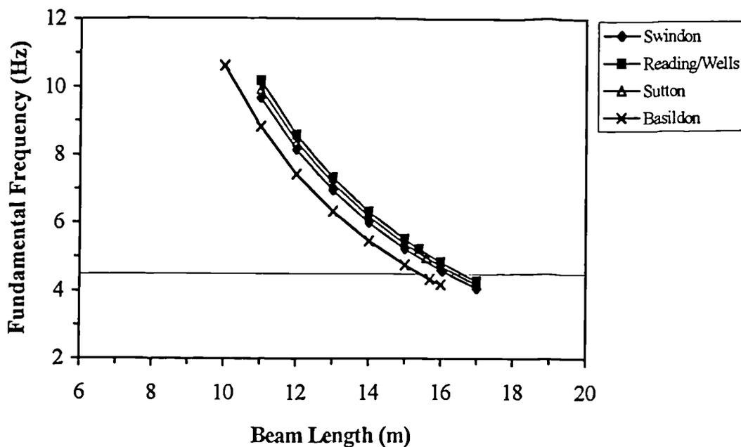
Figure 4.22: Frequency vs Beam Length
