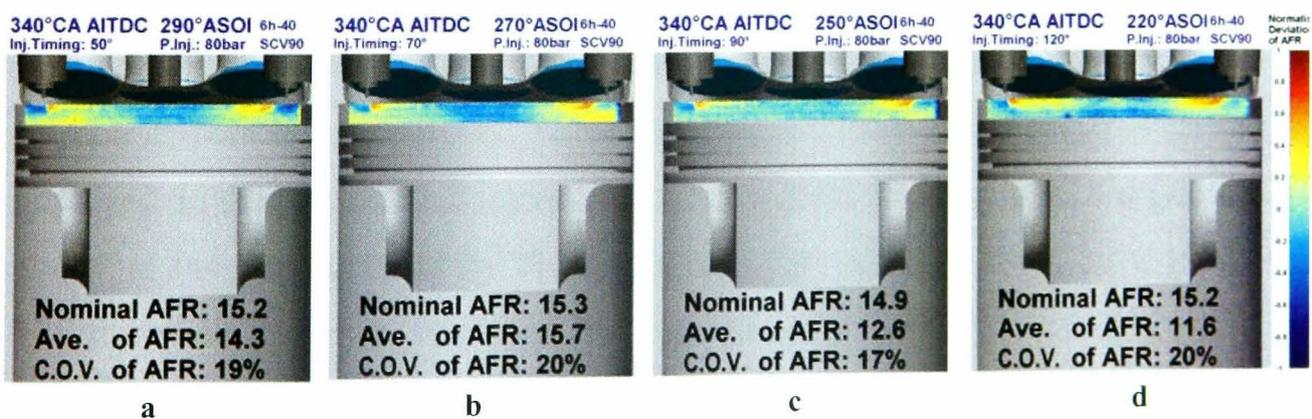
Figure 5.17: Two-dimensional deviation of air/fuel ratio (AFR) distribution at  $340^{\circ}\text{CA}$  ( $20^{\circ}$  before compression TDC) of the 6-hole injector at injection timings of (a).  $70^{\circ}$ , (b).  $90^{\circ}$  and (c).  $120^{\circ}\text{CA}$ .
