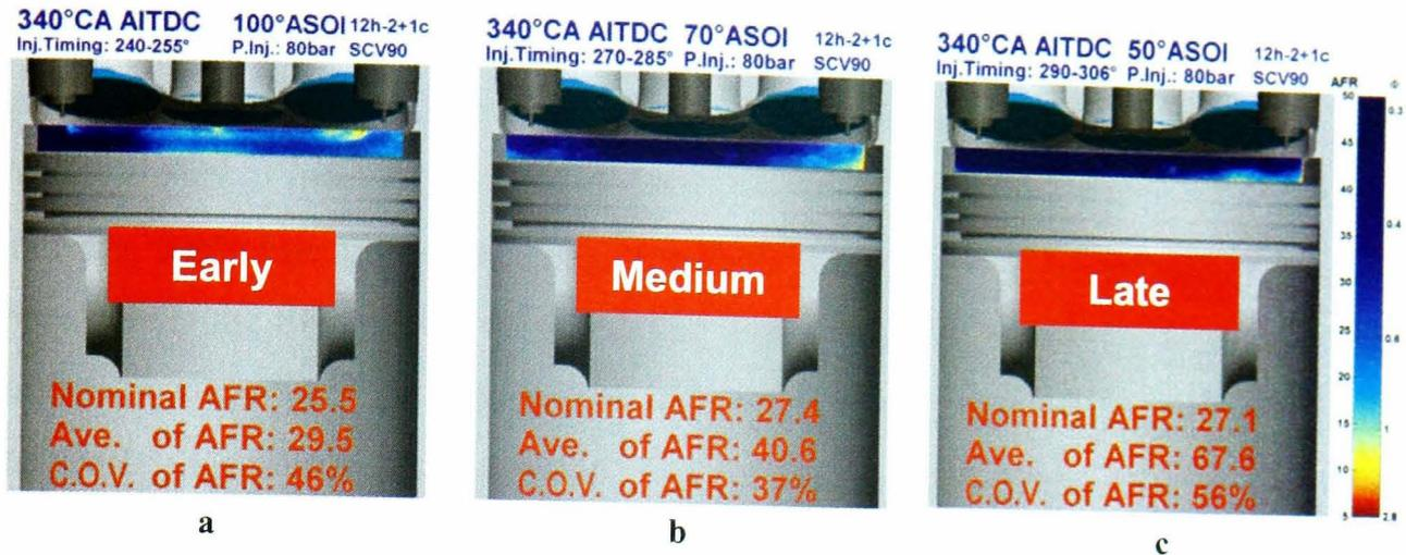
**Figure 5.33:** Two-dimensional AFR distribution for the 12-hole injector at double-injection strategy. Injection timings of (a). 240-255°CA, (b).270-285°CA and (c). 290-306°CA at 80bar injection pressure and 1,500rpm.
