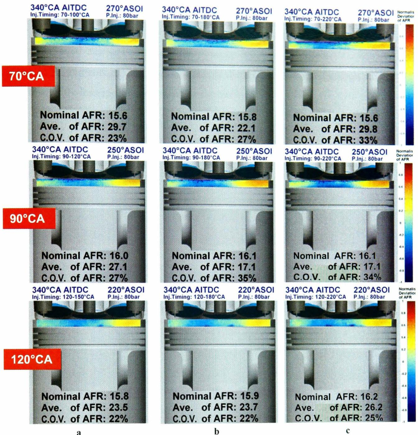
**Figure 5.20:** Two-dimensional deviation of air/fuel ratio (AFR) distribution at 340°C AITDC (20° before compression TDC) of the 6-hole injector at double-injection strategy. The timing of the first injection in the sequence is set at 70°C A (top row), at 90°C B (middle row) and at 120°C C (bottom row). The second injection timing is placed at (a). 30°CA after the start of the first injection event, (b). 180°CA, or bottom dead centre and (c). 220°CA, timing at which inlet valves have closed.
