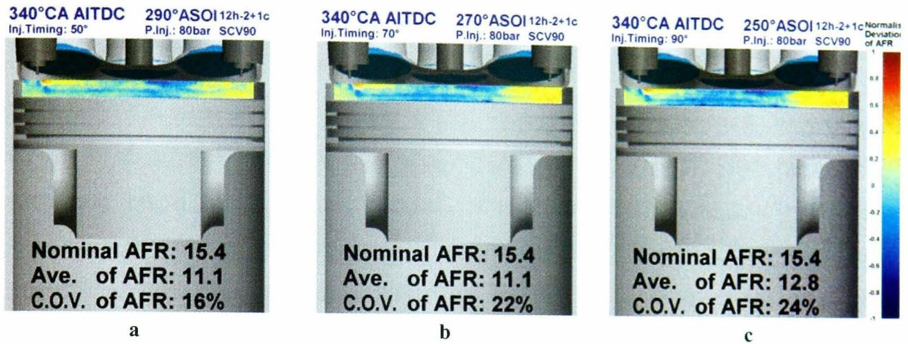
Figure 5.16: Two-dimensional deviation of air/fuel ratio (AFR) distribution at  $340^{\circ}\text{CA}$  ( $20^{\circ}$  before compression TDC) of the 12-hole injector at injection timings of (a).  $50^{\circ}$ , (b).  $70^{\circ}$  and (c).  $90^{\circ}\text{CA}$ .
