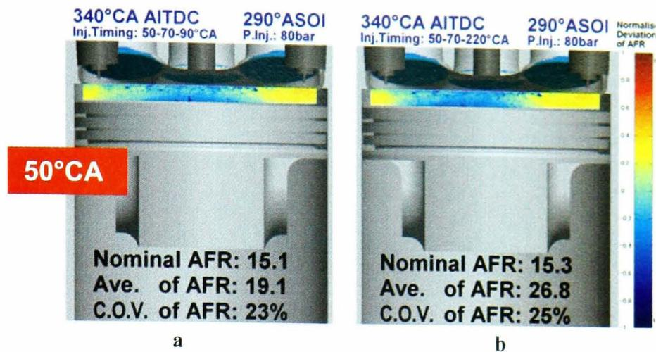
**Figure 5.19:** Two-dimensional deviation of air/fuel ratio (AFR) distribution at 340°C AITDC (20° before compression TDC) of the 12-hole injector at triple-injection strategy. The timing of the first injection in the sequence is set at 50°C A, the second at 70°C A and the third injection timing is placed at (a). 90°C A and (b). 220°C A, timing at which inlet valves have closed.
