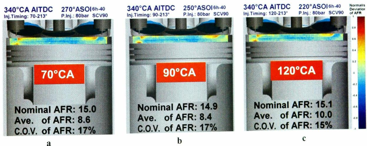
**Figure 5.24:** Two-dimensional deviation of air/fuel ratio (AFR) distribution at 340°C A (20° before compression TDC) of the 6-hole injector at double-injection strategy. Injection timings of (a). 70-213°C A, (b). 90-213°C A and (c). 120-213°C A.
