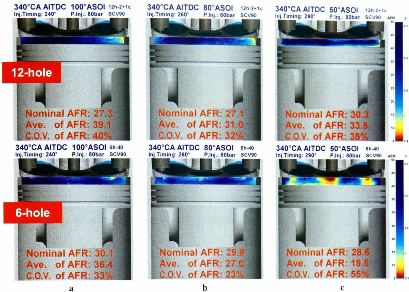
**Figure 5.32:** Two-dimensional AFR distribution for the 12-hole (top row) and the 6-hole (bottom row) injectors at injection timings of (a). 240°CA, (b).260°CA and (c). 300°CA at 80bar injection pressure and 3,000rpm.
