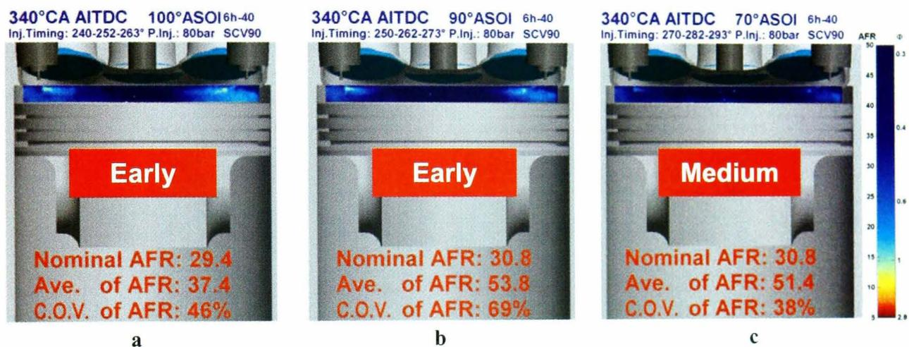
**Figure 5.35:** Two-dimensional AFR distribution for the 6-hole injector at triple-injection strategy. Injection timings of (a). 240-252-263°C AITDC, (b).250-262-273°C AITDC and (c). 270-282-293°C AITDC at 80bar injection pressure and 1,500rpm.
