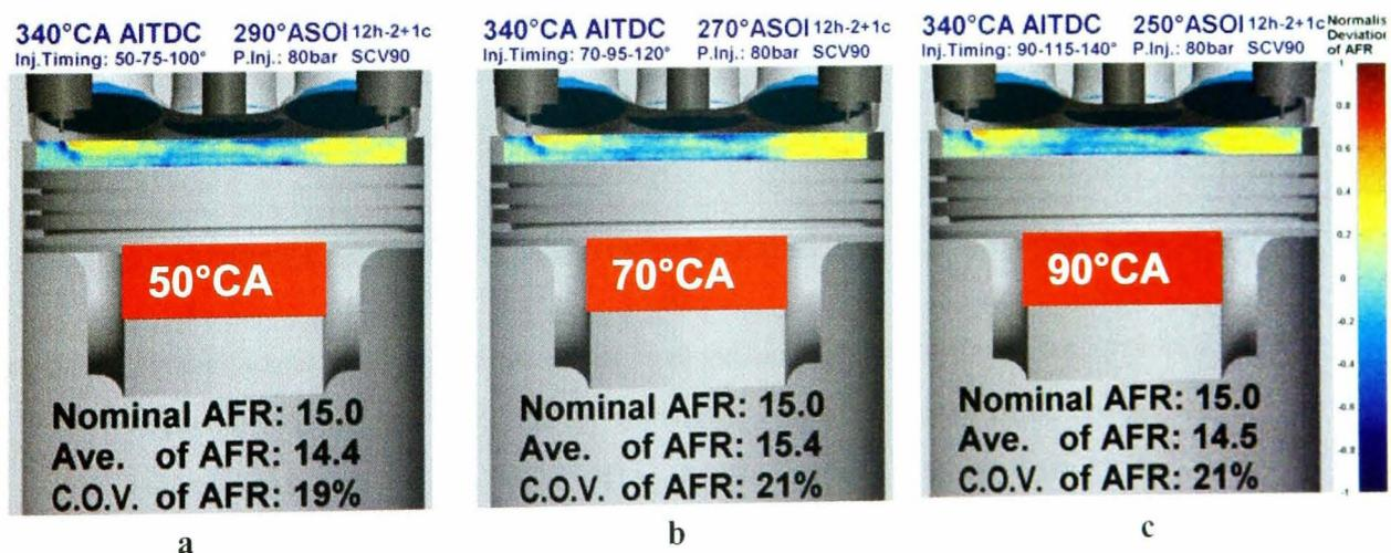
**Figure 5.23:** Two-dimensional deviation of air/fuel ratio (AFR) distribution at  $340^{\circ}\text{CA}$  ( $20^{\circ}$  before compression TDC) of the 12-hole injector at triple-injection strategy. Injection timings of (a).  $50\text{-}90\text{-}120^{\circ}\text{CA}$ , (b).  $70\text{-}110\text{-}140^{\circ}\text{CA}$  and (c).  $90\text{-}130\text{-}160^{\circ}\text{CA}$ .
